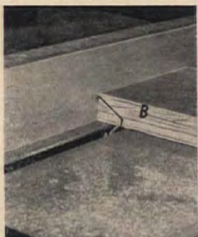
2. SAW IS returned to 0 degrees and lowered to clean out cut on piece "B". Fence is still used as support.
