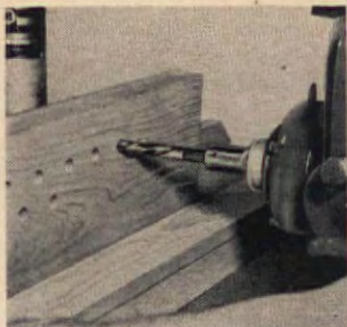
It's a HORIZONTAL DRILL . Direct power drive and radial arm lets you bore at any angle for perfect fits in dowel work.
