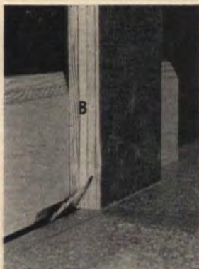
1. AFTER SETTING strip "B" vertically against face on rip fence to make diagonal cut at 30°, reset saw to 0° to make second cut.
