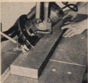
It's a TILT ARBOR SAW . Out-modes every table saw. You move the saw, not the lumber, when you change the type of cut.
