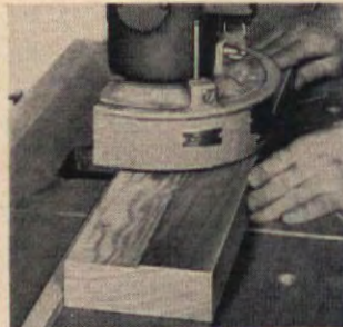
It's a SURFACER . Rotary planer tool fits directly on motor spindle...smooths out rough lumber, gets it ready for sanding.
