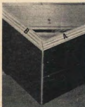
4. MITER JOINT fits perfectly when cut and sanded as described in the text.
