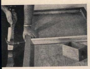
2. Fit a piece of 2" x 2" across center bottom of seat. Fasten with glue and screws: drill for screws through top of seat into cross piece. Countersink screws. Secure ends to seat frame by driving 10d nails through the center of frame into cross piece.
