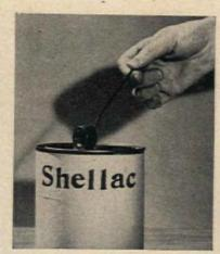
Dip nuts in thinned shellac before you screw them onto the bolt. It will help keep a nut from becoming rust-frozen in place. A drop of shellac on the bolt threads helps keep the nuts from loosening. Shellac won't prevent you from removing nut easily.
