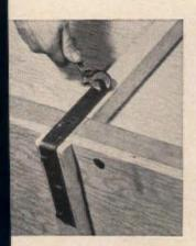
Drill holes for 5 carriage bolts h back. Glue and screw 1" x 3" races to center and sides of ack. Screw back to bottom ith angles to check overall fit.
