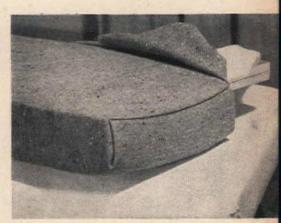
11. Brush coat of glue on back between braces; cover with cotton batting equal to thickness of braces. Pull fabric up and over pad. Fold corners. Trim, tuck in and stitch sides at back edge. Screw back to seat with angle brackets. Fold fabric under seat, pull taut, tack, press.
