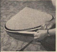
4. After you trim off the excess material, edge of the shade can be finished either by lacing with plastic or covering with cloth adhesive tape. If you use tape, first place temporary strip of masking tape around edge of shade as guide line. Remove this tape after the permanent tape is on.
