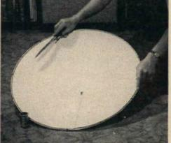
2. Form the cone by overlapping cardboard and holding it temporarily with masking tape. Bottom of shade should measure two feet in diameter to fit 24" wire lamp shade ring. Mark correct position for overlap, then tape and glue it permanently in place. "Feather-edge" the back sides of the illustration board so that seam will be less noticeable.
