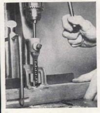
Mortising attachment cuts square holes used for good wood joints. Special fence has hold-down to hold work firmly on table. Depth gauge controls depth of cut
