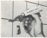
Rubber-base adhesive—best for fastening to smooth surfaces like metal, tile, glass; is ready to use from tube. Glues most materials, needn't be clamped, but it won't stand heat, or extreme stress
