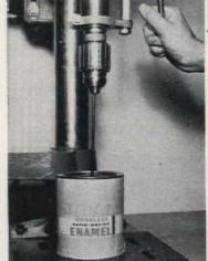
When working with short lengths of material, make sure material is held firmly in place. Use "C" clamps if you don't have a vise. To avoid marring drill table, use a wood block under work, and set depth of stroke so drill stops short of table
