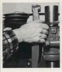
It's important that you operate the drill at the correct speed for each accessory. Instruction book lists correct speeds. Shift belt on pulleys for right speed
