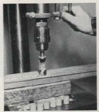
A plug cutter is simply a hollow drill to cut out plugs to hide and cover screw heads. You can use it to cut small dowels by cutting into wood lengthwise
