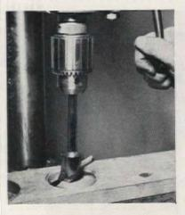
Use adjustable boring tool shown to drill large holes in wood. Drill a small pilot hole first to guide drill. Clamp work securely and operate drill at low speed
