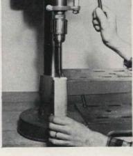
To drill end of long piece, swing drill press head out over floor and clamp work to side of bench. Special wood bits cut faster and cleaner in wood
