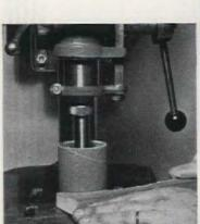
Use sanding drums of different sizes for edge sanding. Use medium speed, and feed work into turning drum. For small work, use small dowel coated with glue and dipped in abrasive grit
