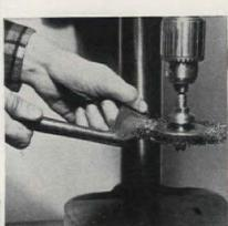
Wire brush can be used to remove rust from tools, cloth buffing wheels to polish metals and plastics, and you can use a cup-grinding wheel for sharpening tools and knives
