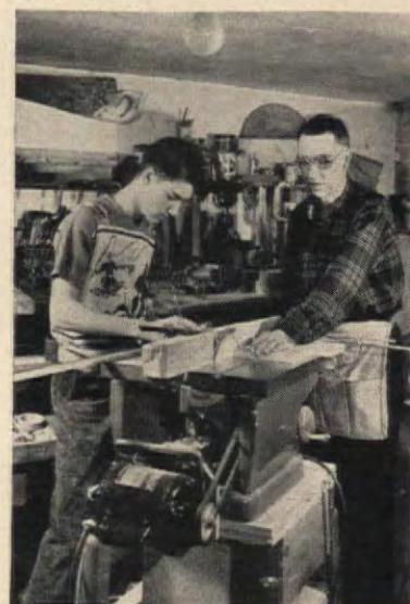
For more accurate edging of boards and strips, here's the jig developed with disk sander attachment on a table saw
