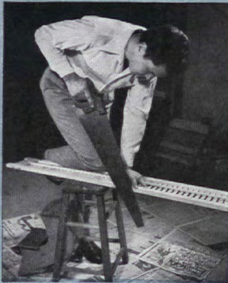
Protruding tenons are sawed off, rabbet is cut on power saw or by hand with a rabbet plane, and ends are trimmed to fit window. Long shutters can be cut in two at rail
