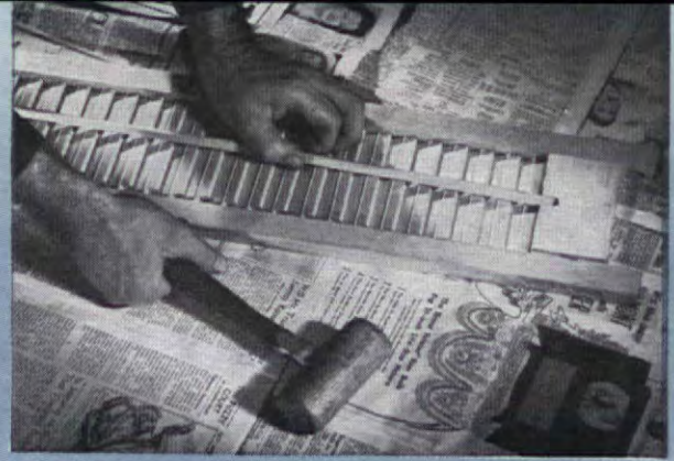
Frame of stiles and rails is assembled loosely, then louvers are fitted in place with a screwdriver or button hook, and the stiles are tapped tightly together
