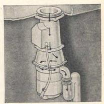
Here's how the Disposall looks and performs. Arrows show how the shredded liquefied waste is carried down the drain.
