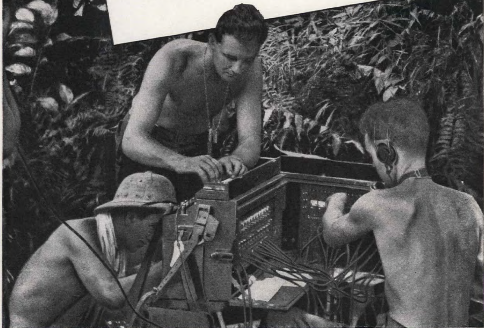
U. S. Army Signal Corps installing switchboard in New Guinea
