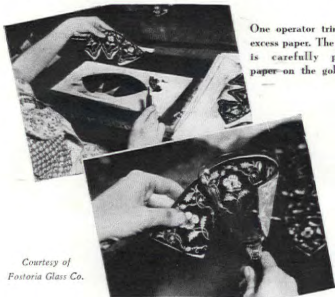
Steps in the process of etching glass: Master etching design engraved on a steel plate. One of these patterns is being filled with an inky wax. A thin strip of paper is then laid on ink and pressed down. Paper is then removed which gives a finished print to be applied to the glass
