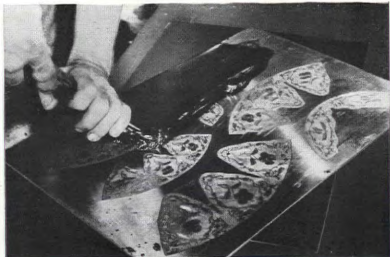
Steps in the process of etching glass: Master etching design engraved on a steel plate. One of these patterns is being filled with an inky wax. A thin strip of paper is then laid on ink and pressed down. Paper is then removed which gives a finished print to be applied to the glass
