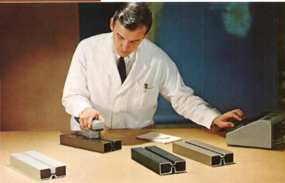
KAWNEER PERMANODIC QUALITY CONTROL in basic alloy, electric input, temperature control and pre-anodic preparation, plus frequent photovolt meter checks, assure close tolerance of color variation. Select from light bronze, medium bronze, dark bronze, or black.
