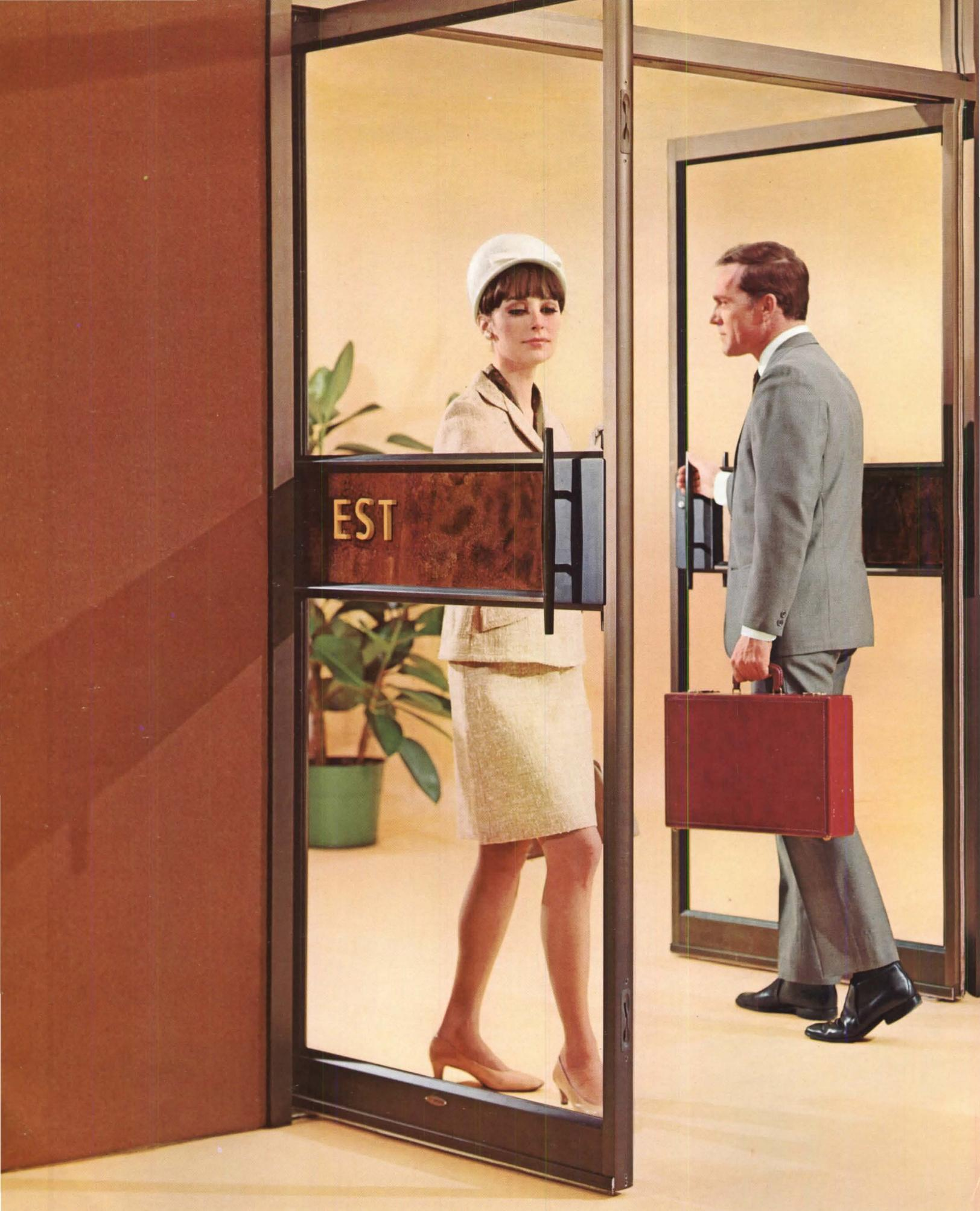
STYLE LEADER 125 ENTRANCE. Unlimited options in center identification panel, using any quarter-inch thickness material . . . wood, porcelain, plastic, glass. Permits customizing of standard doors. Each 125 has weathering on all 4 sides. Top and bottom locking bolt eliminates cut-out in door stile. Closer concealed in transom.
