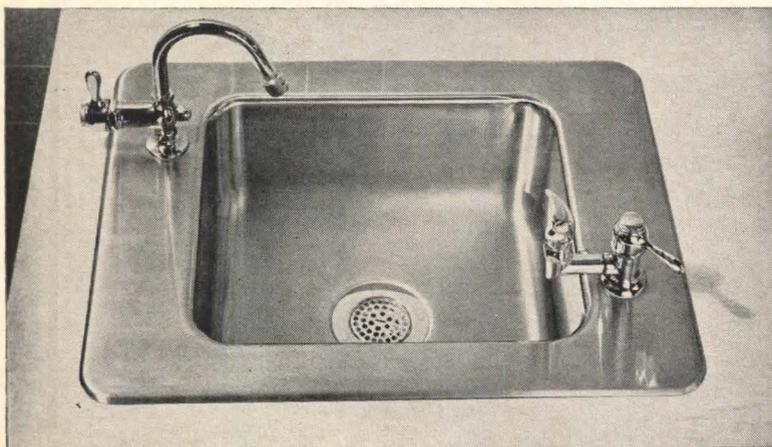
**Classroom Counter-Top Fountains** Complete "self-rimming" type pre-assembled for easy installation. Stainless steel receptor has push-button-operated, two-stream projector with automatic stream control. Goose neck glass-filler faucet optional. Also available in porcelain-enameled cast iron.
