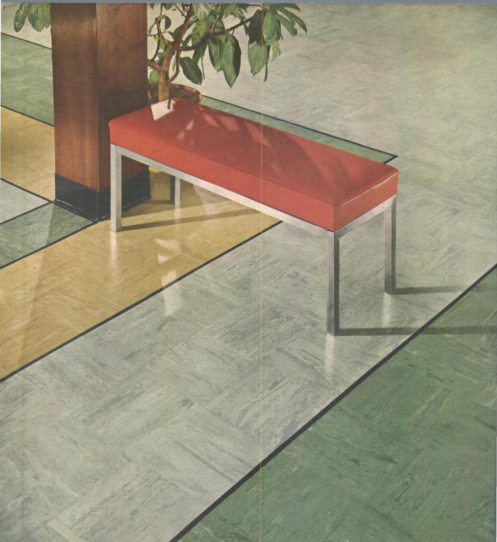
Low-cost Kentile® Architectural Marbles Vinyl Asbestos Tile comes in two thicknesses:  $\frac{3}{2}$ " and  $\frac{1}{8}$ ." Nine colors. Shown above with  $\frac{1}{2}$ " feature strips.
