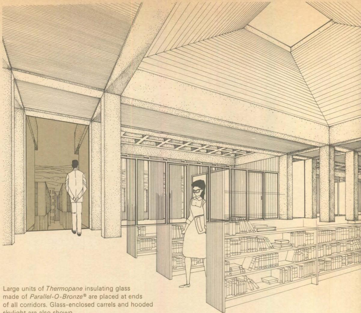
Large units of *Thermopane* insulating glass made of *Parallel-O-Bronze*® are placed at ends of all corridors. Glass-enclosed carrels and hooded skylight are also shown.
