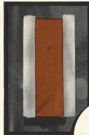
LP<sup>®</sup> polysulfide base sealant after 30 cycles in Joint Movement Simulator. Like new.
