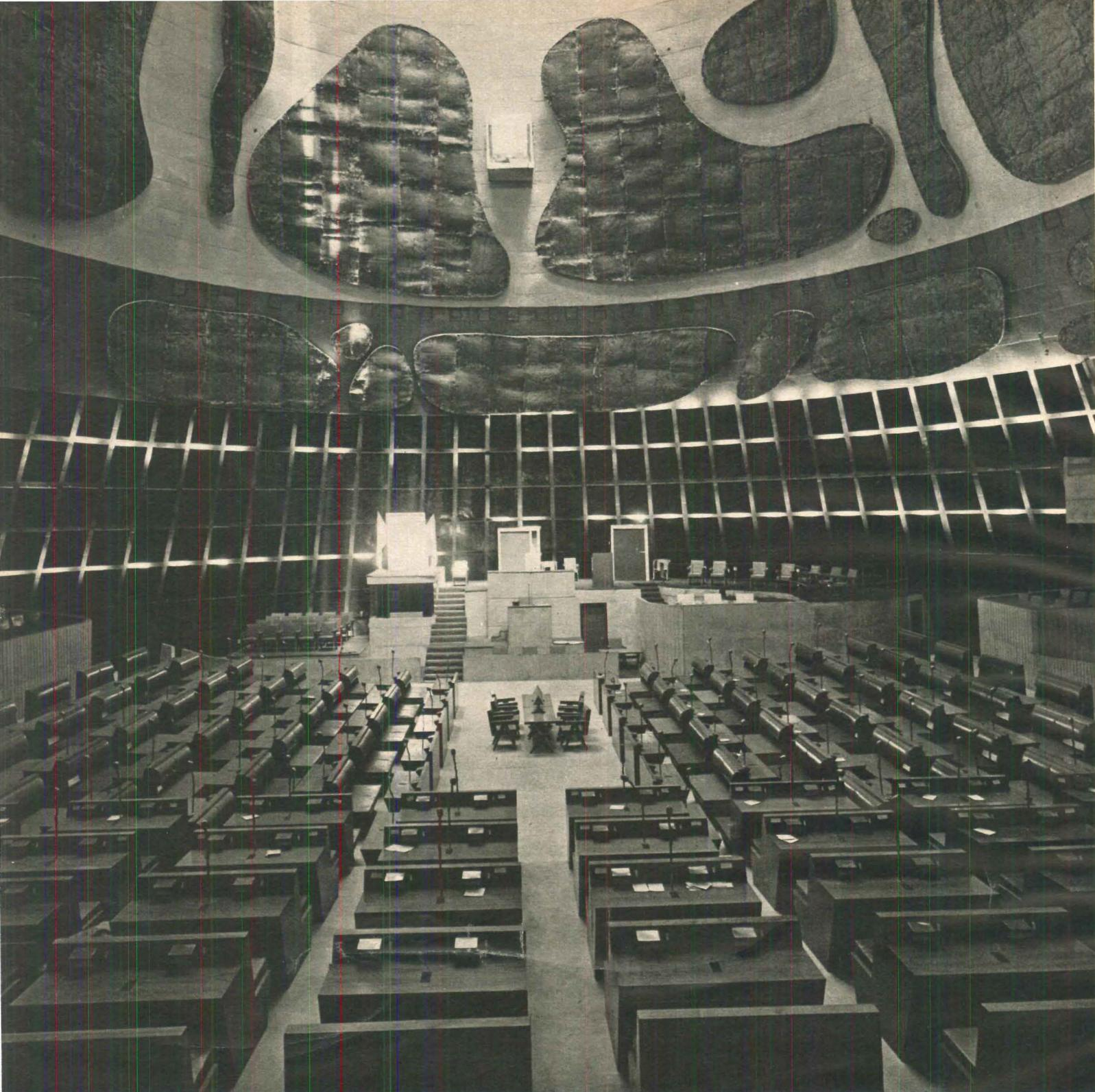
*Hyperbolic Assembly Hall is lit through a great skylight at the top of its funnel shape. Funnel contains ventilation and sound equipment.*
