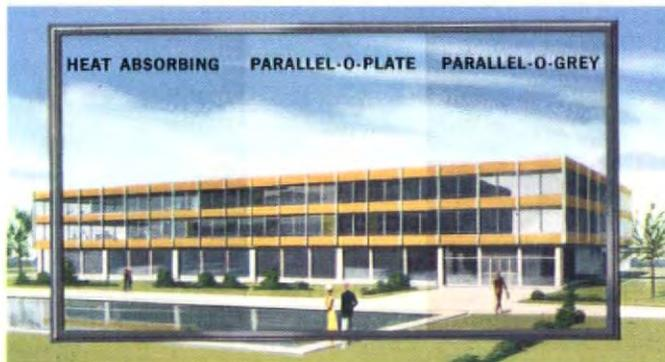
**THREE KINDS OF PLATE GLASS**—To achieve clear vision from inside and a richer appearance on the outside, use twin-ground *Parallel-O-Plate®* Glass in windows. For control of sun heat and glare, use *Parallel-O-Grey®* or Heat Absorbing Plate. *Parallel-O-Grey* is neutral grey in color. Heat Absorbing Plate is pale bluish-green. Both effectively reduce transmission of sun heat to keep interiors cooler, but *Parallel-O-Grey* is more effective in reducing glare.
