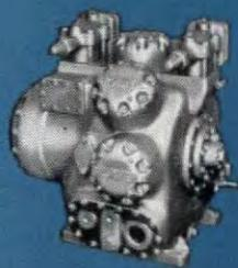
Brunner-metic units are available in the following series: air cooled, water cooled, combination air-and-water cooled, capillary tube, truck and remote condenser system models. Compressor capacities range from ¼ H.P. through 15 H.P. Bolted construction permits easy dismantling for servicing. Suction gas cooled motor contributes to higher efficiency and longer life. Crankshafts are dynamically and statically balanced for smooth operation.
