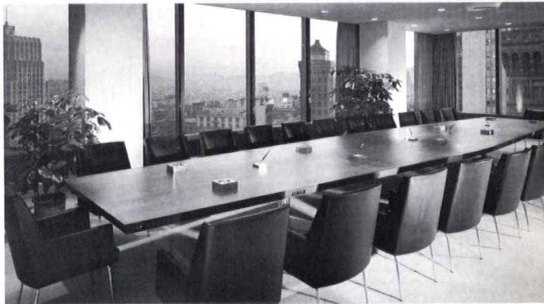
The board room is a bright and cheerful place to work because of the wide expanse of window area. SOLEX heat-absorbing glass used here absorbs about 50% of direct solar radiation and reduces glare.
