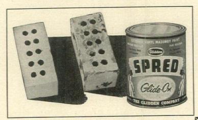
Four-Year Exposure Test of bricks above shows superior durability of SPRED GLIDE-ON—new exterior masonry finish for stucco, brick and asbestos shingles. Brick at left painted with SPRED GLIDE-ON did not peel, chip or flake in four years.
