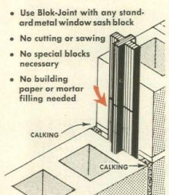
BLOK-JOINT is a "cross-shaped" rubber extrusion which greatly simplifies the construction of masonry wall control joints. It can be used with any standard metal sash block! Made of "100 year life" rubber, it forms a secure interlock and adds stability to the wall.
