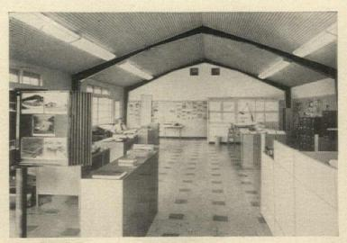
Spacious clear-span interior of Butler steel building, handsomely and economically modified, provides post-free space for greatest usability, convenient arrangement of office equipment.
