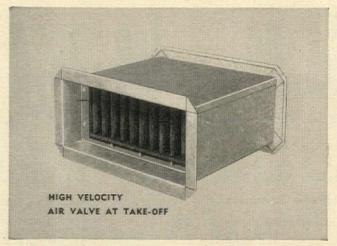
One Uni-Flo High Velocity Valve can serve several diffusers when installed at a low velocity branch duct take-off from a high velocity trunk duct. Or a "package" is available, consisting of an air valve, sound control-chamber, and single diffuser.
