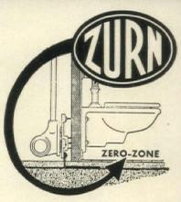
The Zurn Zero Zone® is created by mounting off-the-floor plumbing fixtures on behind-the-wall ZURN SYSTEMS. This permits the highest degree of rest room sanitation to be attained and maintained. All major plumbing manufacturers make fixtures to fit this system.
