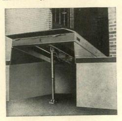
the ramp as much as 15" from dock level to follow the truck bed. To prevent any sudden drop of the ramp when the truck pulls away, an automatic safety switch locks the ramp instantly in place. When not used for loading, the Trans-O-Matic may be set at dock level for cross-over traffic or for use as a storage platform. Five cast steel hinges, welded to the mounting plate, provide continuous support at the dock edge.
