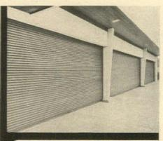
Typical installation, Cookson Standard Type FC 29'x 13' Steel Rolling Doors.
