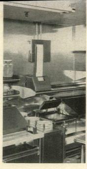
2. Order, transmitted by wire, appears simultaneously on roll of paper in kitchen. Grille below is for hot snacks; full hot meals are elevatored up from another cafeteria kitchen.
