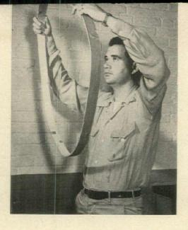
based flooring is as resilient as hardwood and will not crack under extreme temperature changes. The waterproof, nonslip composition is resistant to alkalis and mild acids. It can be used in its natural gray state or dressed up with pigment for applications in hospital rooms, school corridors and auditoriums, and offices. Shipped as two components—liquid rubber and cement powder—Laticrete is mixed on the
