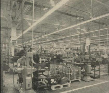
Day-Brite CFI-10 (Comfort For Industry) with 10% upward lighting. Ceiling contrasts are washed out and greater visual comfort assured.
