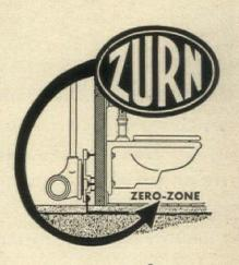
The Zurn Zero Zone is created by mounting off-the-floor plumbing fixtures on ZURN SYSTEM behind-the-wall fittings and carriers. This permits the highest degree of rest room sanitation to be attained and maintained. All major plumbing manufacturers make fixtures to fit this system.
