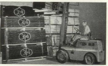
10. PACKAGING ECONOMY—Wheeling's "Engineered Metal Lath Package"—lifts of 500 sheets in 50 10-sheet bundles—increases storage space, saves handling, counting and identifying time. Provides flatter sheets with truer corners.
