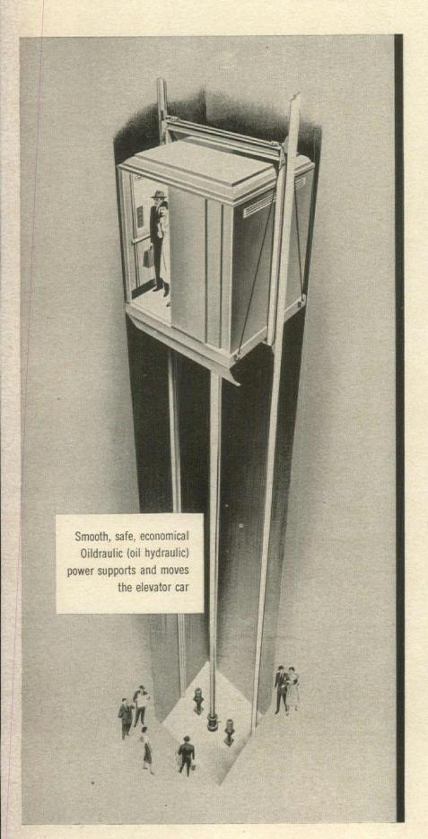
Rotary Oildraulic Elevators, moved and controlled by oil under pressure, have definite architectural and operating advantages for modern buildings.
