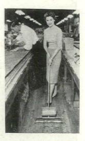
the 10%"-wide rotary Sweeperette. Selling for \$34.50, this 5-lb. light-duty unit operates like a carpet sweeper. Metal accumulated on its tube is pushed off easily with a neoprene wiper ring. Super Sweepers produced in three strengths for use at different speeds range in width from 35½" to 71½" and in price from \$303 to \$765. Manufacturer: Eriez Manufacturing Co., Erie, Pa.
