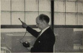
A similar test using a portable pyrometer confirmed the findings of the test using thermocouples by showing the same 14 degrees lower temperature on the roomside surface of the 80-F glass block.
