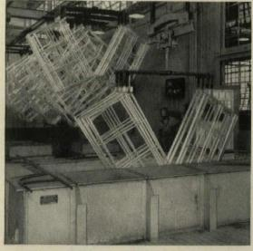
Super Hot-Dip Galvanizing is done in Fenestra's own special plant-the only one of its kind in America. A uniform coating is assured by complete immersion in molten zinc.
