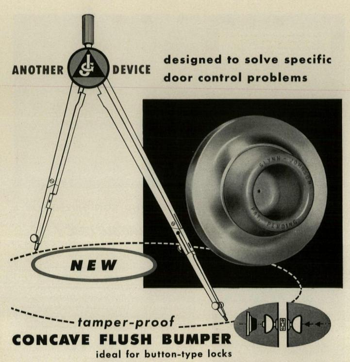
Has no visible mounting screws . . . uses hidden method of attachment. Solves problem of unauthorized removal of bumper or rubber in public buildings. Concave bumper permits knob to strike without damaging or engaging button-type lock mechanism.
