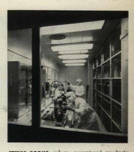
STERILE ROOMS, where parenteral products go into vials for market, are supplied with micronite-filtered air from sanitary plenum above, achieving higher degree of sterility than many hospital operating rooms.
