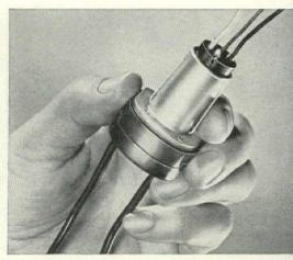
Remote-Control Relay operates on 24 volts—does the actual switching of the higher voltage. Rated 10 amps at 277 volts. U. L. approved.
