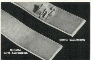
BEND TEST shows why Fenestra Steel Windows are called Super Hot-Dip Galvanized. When two pieces of galvanized steel are bent, then straightened, some types of galvanizing crack open, leaving the steel vulnerable. The Fenestra piece stays protected.
