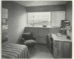
Rooms have many built-ins, from bulletin boards to medicine chests. Under window is continuous convector with adjustable shutter to permit a degree of temperature selection. Towel-drying racks are recessed into face of convector.
