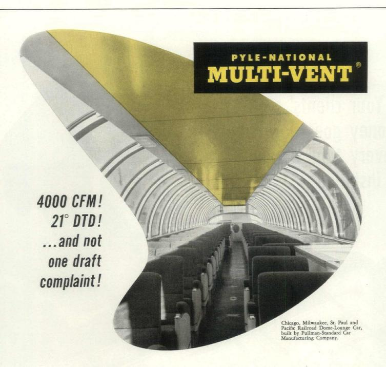
To counteract the tremendous amount of radiant solar heat and avoid hot, humid "greenhouse" conditions in the glass dome sections of these new railway cars, the maximum cooling load calls for 4000 cubic feet of air per minute at 21 degrees below the desired comfort zone temperature. Introducing this very large volume of cold air into such a confined low ceiling area without setting up cold drafts and a high noise level was possible only with the use of Multi-Vent air diffusing panels.
