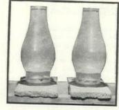
Prepare two slabs of mortar, one with Brixment and one with ordinary cement-and-lime mortar. After mortars have hardened, seal a lamp chimney to each of the mortar slabs, using wax or candle grease, and fill with water.
