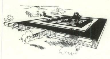
Science building will use flexible plan and economical construction of a small factory with a court cut out of it.
