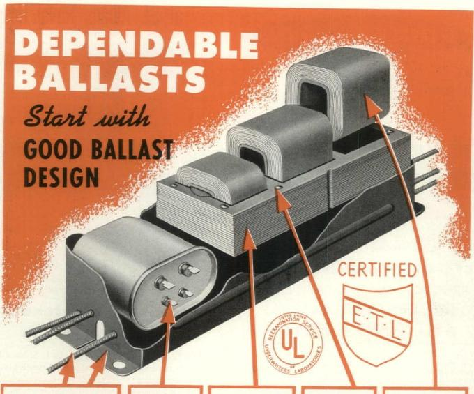
All Advance core and coil assemblies are completely enclosed in moisture resisting, dust-proof containers, die-formed or drawn from heavy gauge cold roll steel, thus affording sturdy, uniform construction. All containers are coated with a rust protecting, lasting black japan finish. Rubber covered cotton braided heat-resistant U. L. approved lead cable is firmly anchored to the coil leads. All external lead lengths are sufficient for easy installation without splices.
