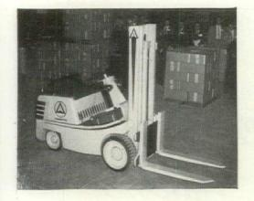
pean sports cars could prove that its newness was more than chassis-deep; indeed, the sleek shell encases a sense-making principle of operation. Gas-engined for rugged service, the Dynamotive has an electrical transmission for a wide acceleration range with minimum power loss. There is no mechanical connection between engine and drive unit, and so no shock load can be transferred from wheels to engine. Transmission gears, hydraulic torque converters, and overdrive mechanisms (all
