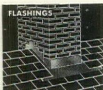
Terne step flashing applied to chimney on slate roof.
