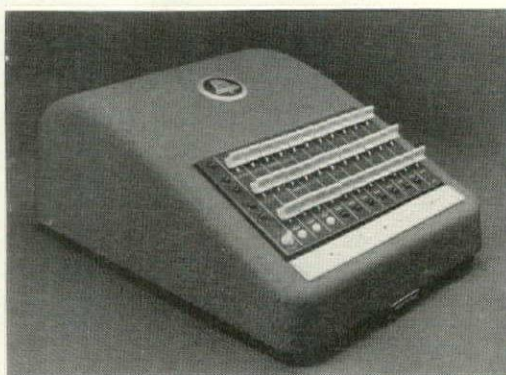
PBX switchboard for Bell Telephone
