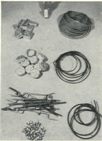
By using low voltage remote control switching equipment pictured at left, the copper and steel items at right were saved in a house having a floor area of 724 sq. ft. (Note size of hand photographs for comparison.)
