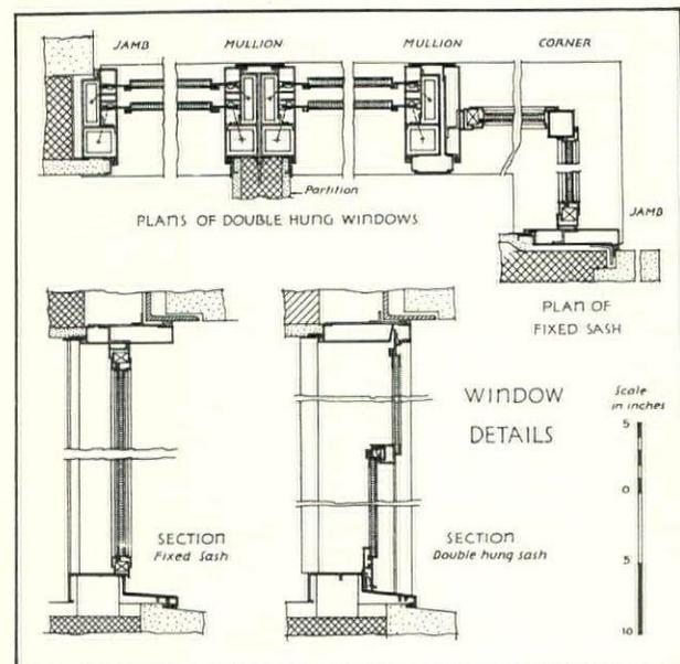
Aluminum was used for most of the windows throughout the building, due to its color, its light weight, its comparative resistance to corrosive stain. These details show the result of designing for a minimum thickness in structural members. This is particularly noteworthy in the case of the banking room windows where mullions are only 1 in. thick
