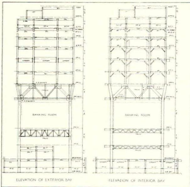
Typical framing diagrams showing the trusses and knee-braces
