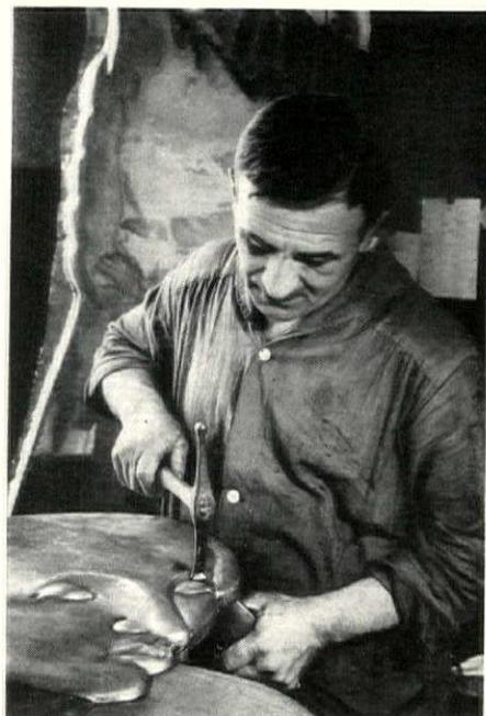
At the right, one of the steps in repoussé work, beating out the form from a flat sheet with a hammer, while holding an iron underneath
