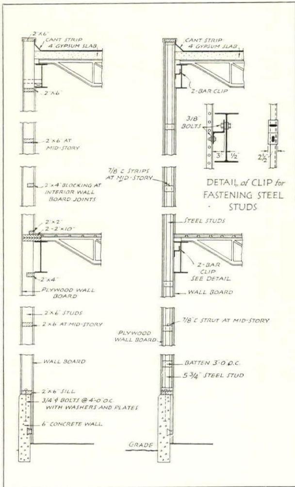
The construction of the Hall of Science is somewhat similar to that of the Administration Building published in the August 1931 issue of *The Architectural Forum*. In the Administration Building the wall membrane was transite; here plywood has been used secured to a stud framing outside of the steel frame. Below are two types of stairways used
