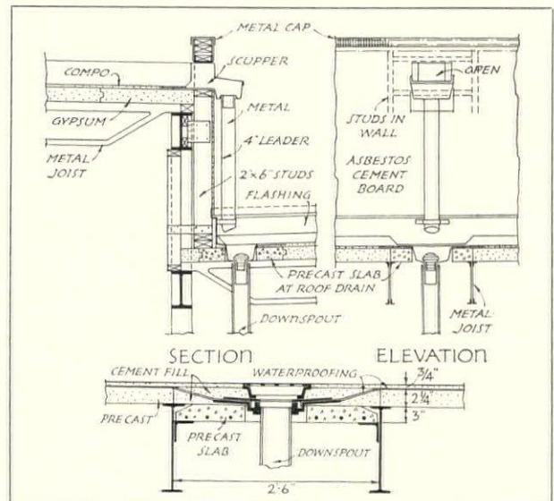
Construction of the roof sumps and parapets. The drawings above illustrate the drainage from one roof level to another
