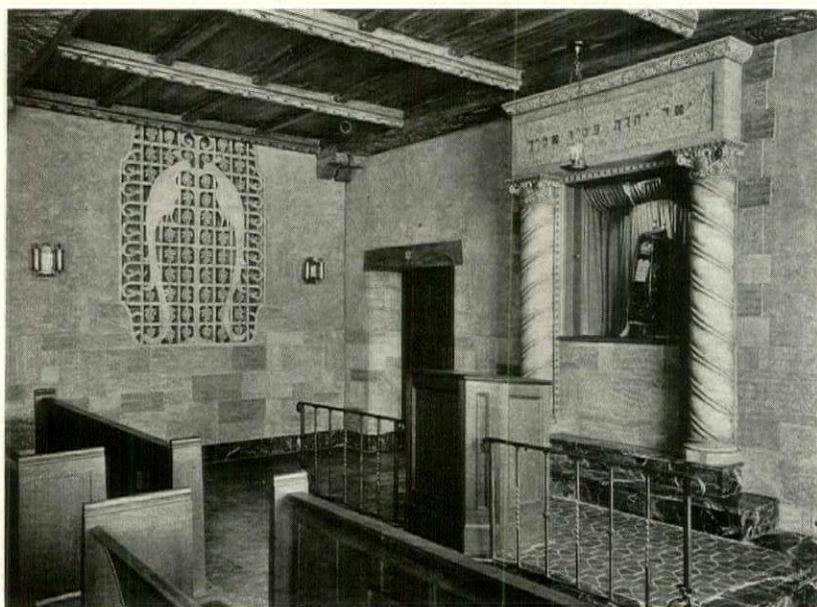
ABOVE is a general view of the auditorium, and at the left, one of the chapel. A similar treatment is employed in both — rough plaster walls with travertine block dado wainscoting and trim, and both ornamented by symbolic painting and carving. The total cost of the building, which has a cubage of 750,000 cu. ft., was \$400,000, or 55 cents per cu. ft.
