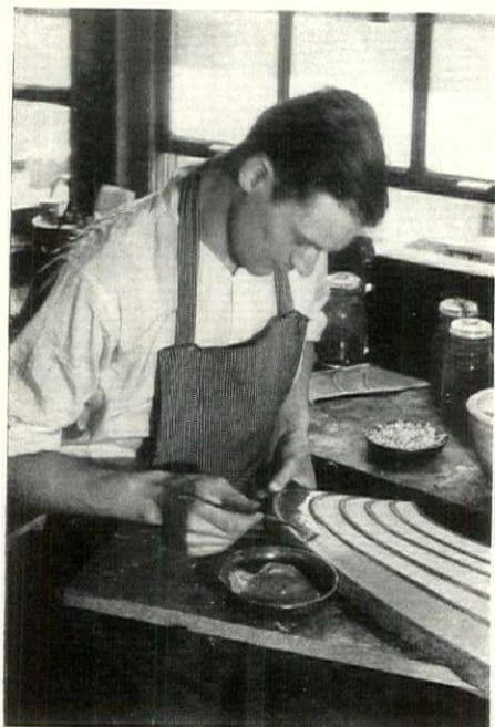
Spreading soft enamel for one of the plaques after the repoussé work had been finished. The enamel is then baked to form a thin glaze
