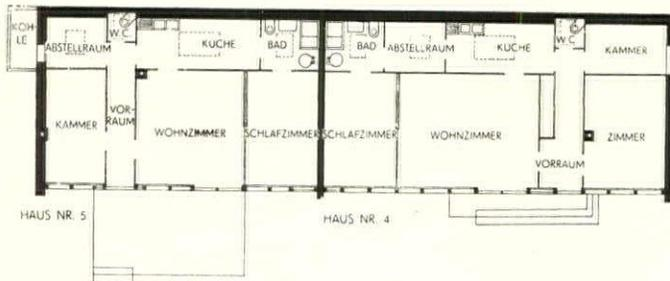
An open type one-story bungalow, designed by Hugo Häring of Berlin. With only two bedrooms, a living room, and the necessary service and storage facilities, an interesting system of ventilation has been worked out as well as a method for quantity production
