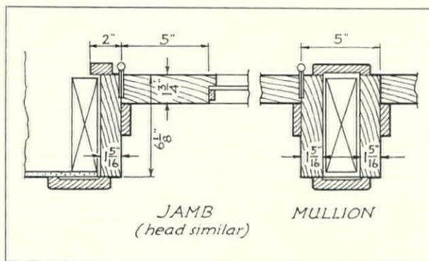
A typical detail of one of the entrance door jambs and mullions. The doors are installed in the stud walls shown in section on the opposite page
