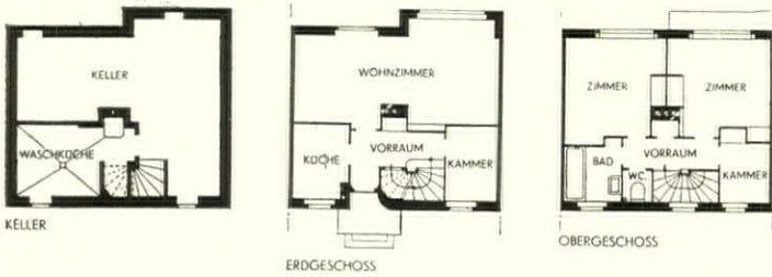
Designed by Oskar Wlach of Vienna, this two-story row house is typical in plan of current housing practice, with a large multiple-use room on the first floor. As is more common abroad than here, the bath and toilet are separate
