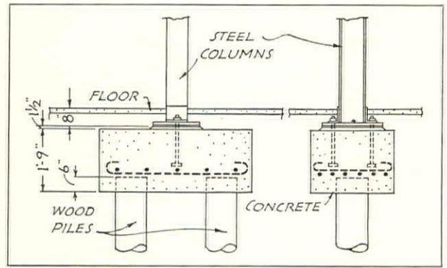
At the left is a view of the interior of the Great Hall showing the method of framing the walls and roof. Most of the structural steel frame is secured by bolts and the joists, secured by clamps to the beams, are stiffened with bridging. The drawing above is typical of the foundation system. Two piles under a concrete footing support the interior columns and one pile only is used beneath the exterior columns
