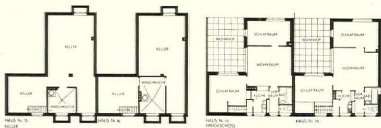
A rather unusual L-shaped bungalow designed by Anton Brenner of Vienna. Simpler in form than almost any other house in the exposition, the cost of construction is remarkably low. The private court for each unit and the grouped service facilities are commendable features of the plan
