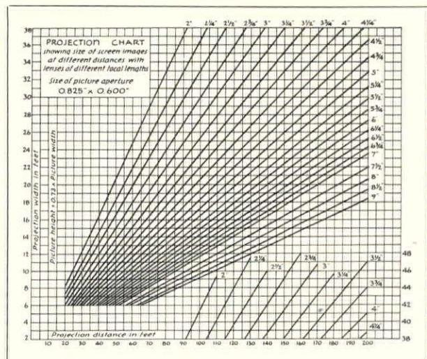
Figure 2. This chart may be used to determine the proper relation between screen width and the projection distance, from which, with a lens of proper focal length, ideal projection may be obtained
