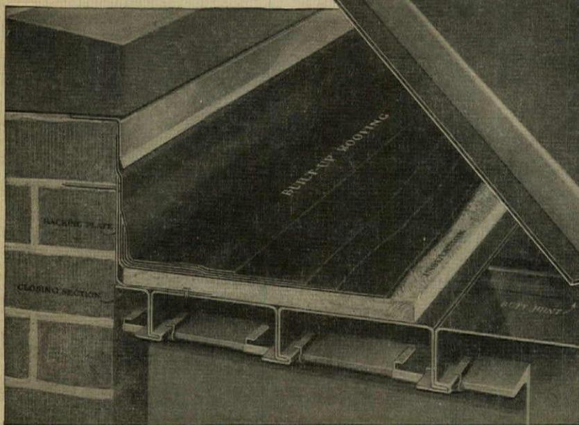
Section Showing Ferrobord Roofdeck, Insulation and Built-Up Roofing
