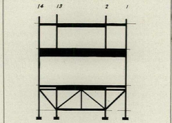
Fig. 2. The large girder and the inverted truss were necessary to accommodate the wide show front shown at the upper left corner of this page
