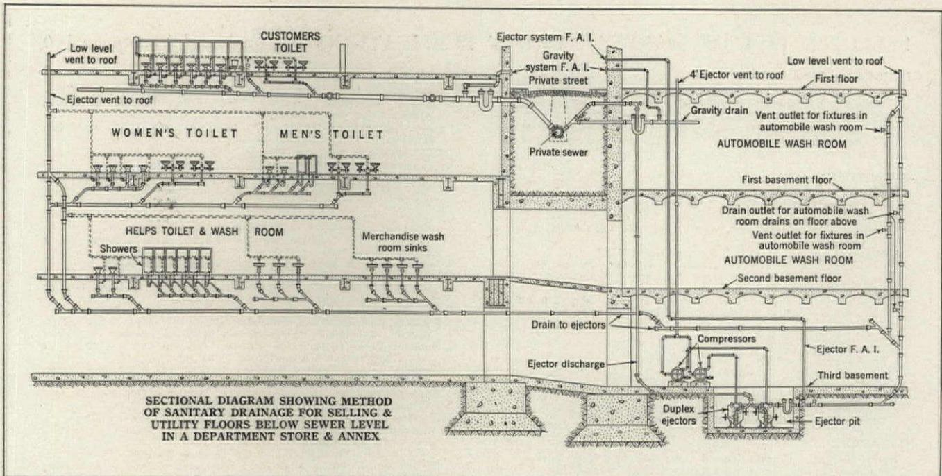
SECTIONAL DIAGRAM SHOWING METHOD OF SANITARY DRAINAGE FOR SELLING & UTILITY FLOORS BELOW SEWER LEVEL IN A DEPARTMENT STORE & ANNEX
