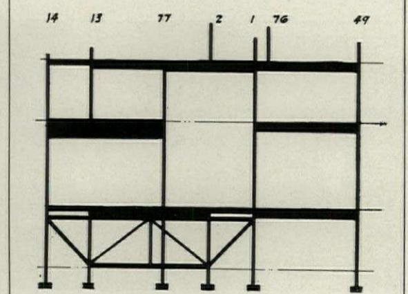
Fig. 3. The alterations in the structural frame shown here were to accommodate the new shop front shown on the preceding page
