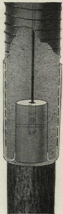
VIRTUALLY a one-piece pile—that is the result obtained by the Raymond Method of joining the timber to the concrete in this type of l-o-n-g pile. It is as perfect in the ground as on paper, as this cut-away section demonstrates.
