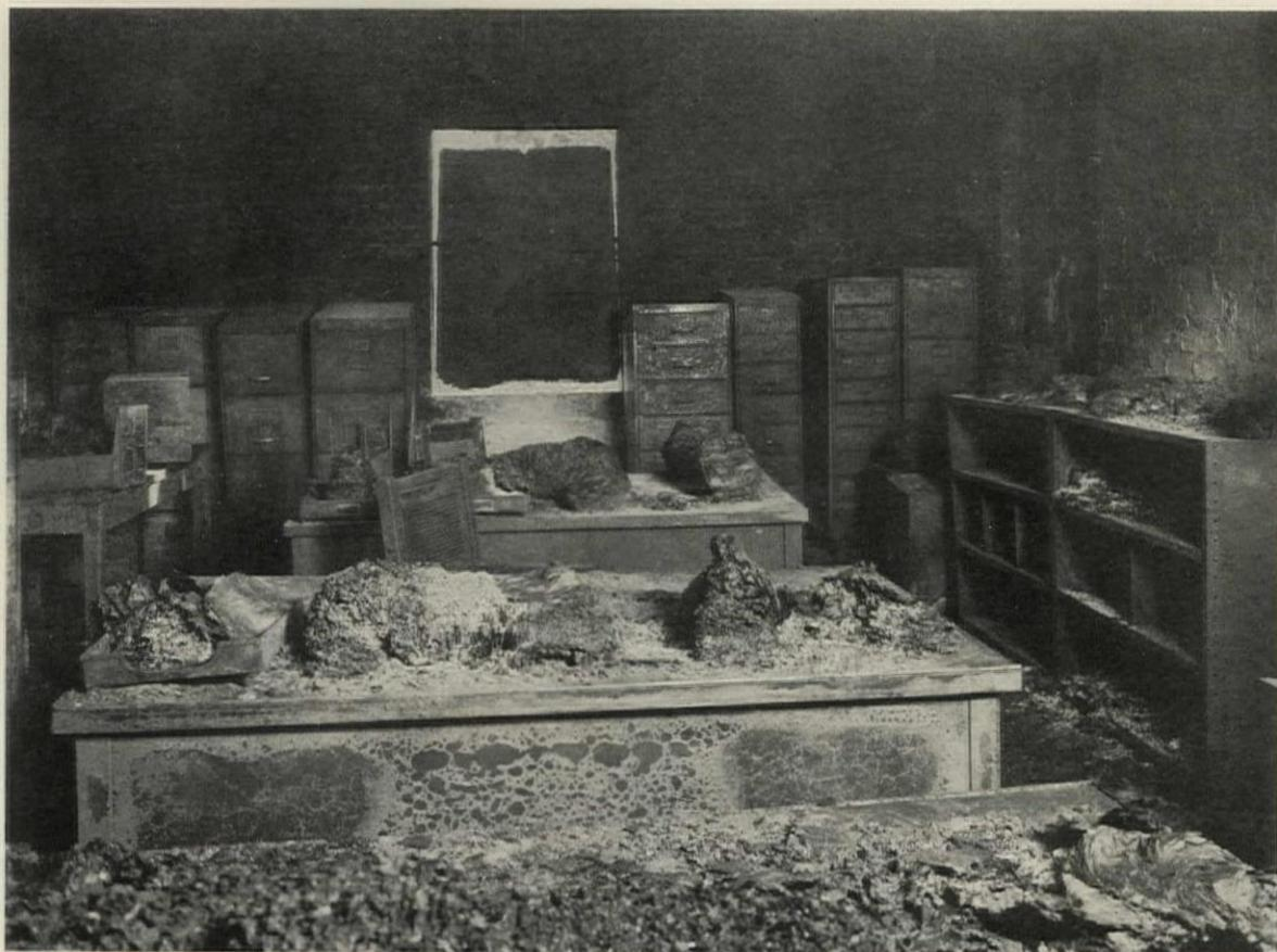
Fig. 6. Metal Furniture on Wood Floor After a Fire With Exposure Start
