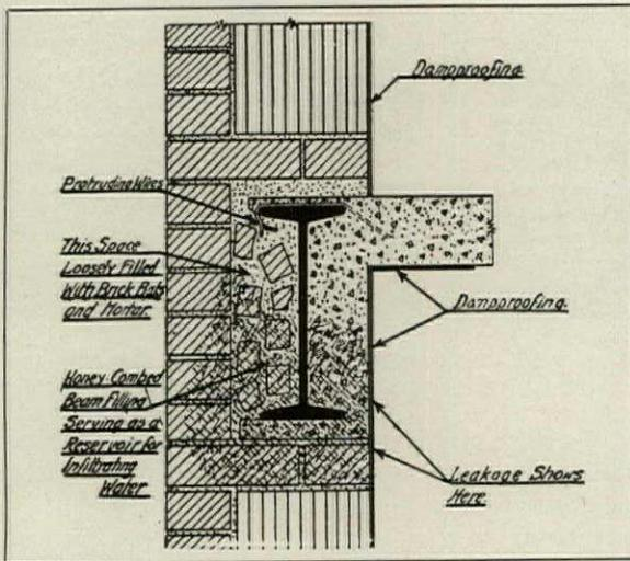
A Typical Spandrel-Beam Construction That Frequently Causes Leakage
