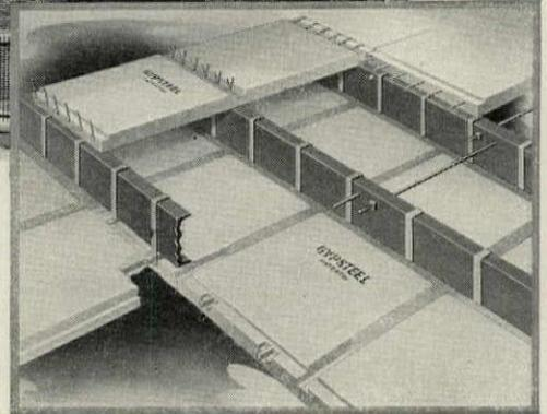
A feature of Gypsteel construction is the flat ceilings, better for sanitation and light reflection.
