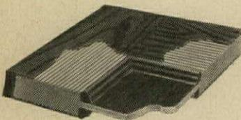
*R-W Compound Key Veneered Doors have laminated stile and rail core construction. Extra heavy sawed veneer is applied by the exclusive tongue and groove method. The result is a combination of beauty and sturdiness that lasts for decades, free from warping, swelling, shrinking, etc.*
