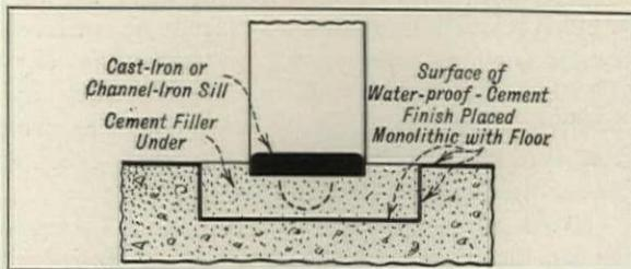
Cement Waterproofing Under a Metal Door Sill
