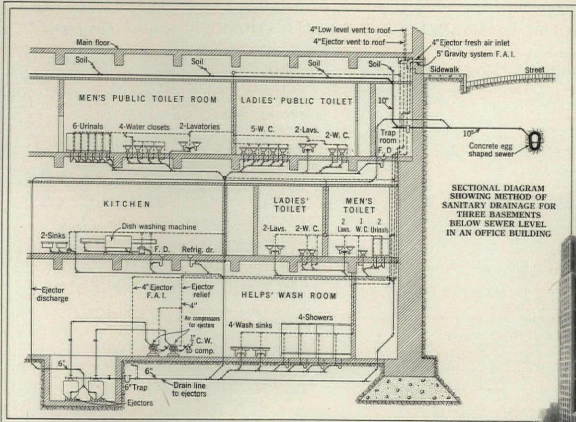
SECTIONAL DIAGRAM SHOWING METHOD OF SANITARY DRAINAGE FOR THREE BASEMENTS BELOW SEWER LEVEL IN AN OFFICE BUILDING
