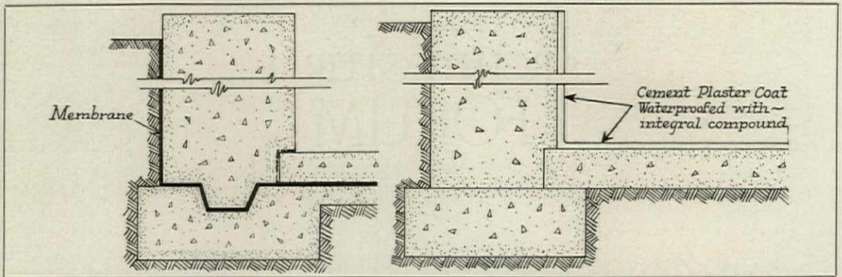
Left: The Membrane Method of Waterproofing Basements Where the Exterior Surfaces of Walls Are Accessible.
