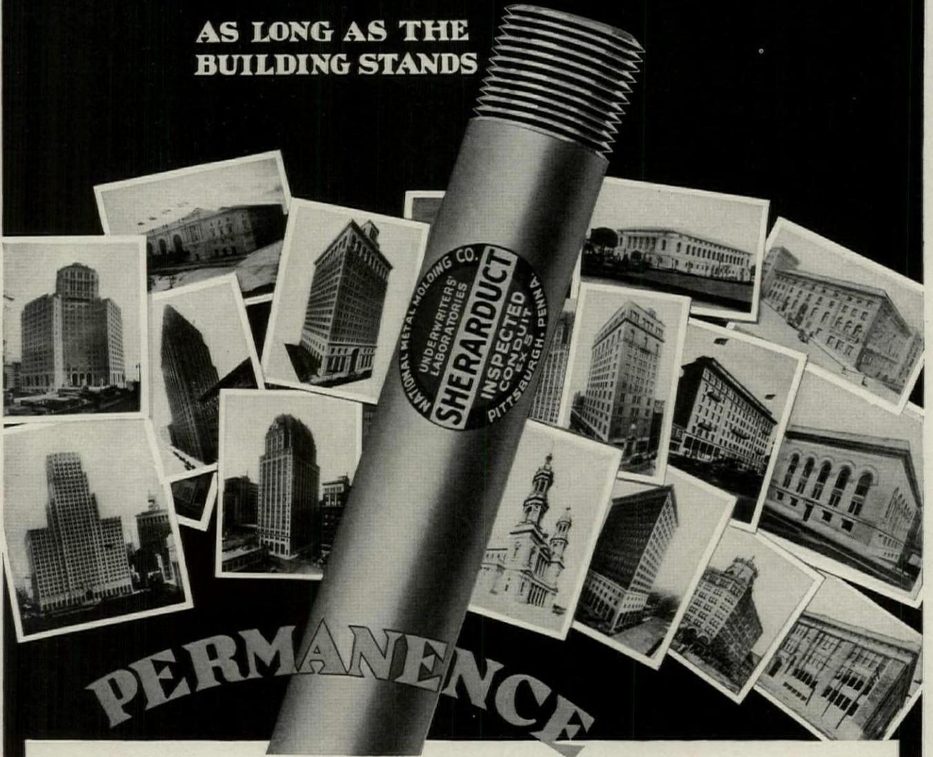
SHERARDUCT CONDUIT is corrosion-proof wiring protection that outlasts the building. Overall zinc impregnation, obtained by Sherardizing, rustproofs the conduit permanently. Enamel baked over inside and outside preserves the zinc under acid conditions.
