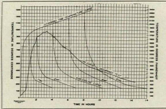
Fig. 3. Standard Furnace Exposure Cooling Curves and Curve From Occupancy Test
