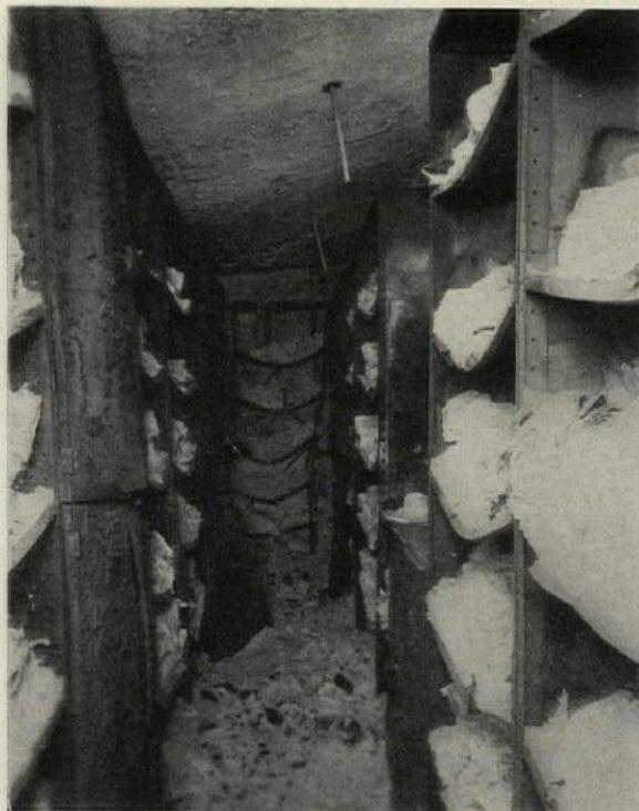
Fig. 8. Metal Shelving, Backed and Partitioned Type, After Fire Test
