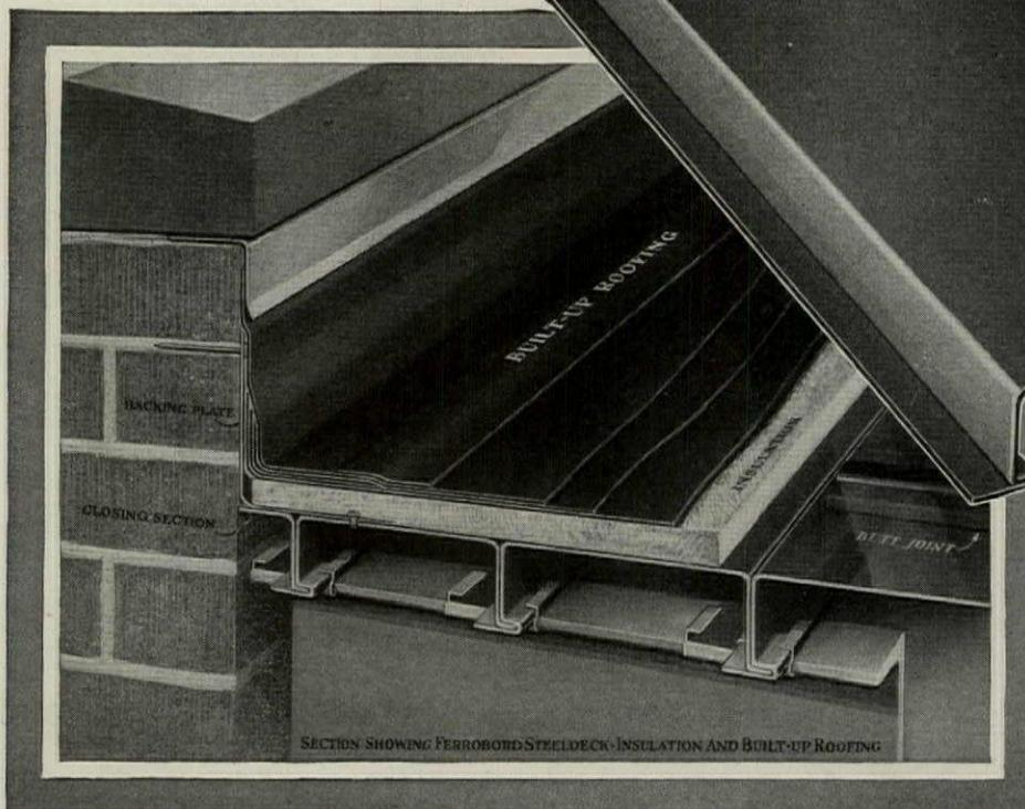
SECTION SHOWING FERROBORD STEELDECK-INSULATION AND BUILT-UP ROOFING
