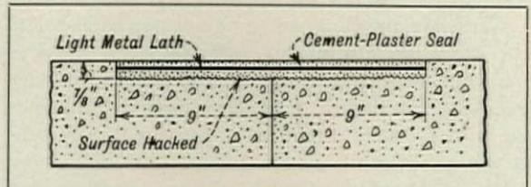
Cement Seal at Joint in Integral Waterproofing
