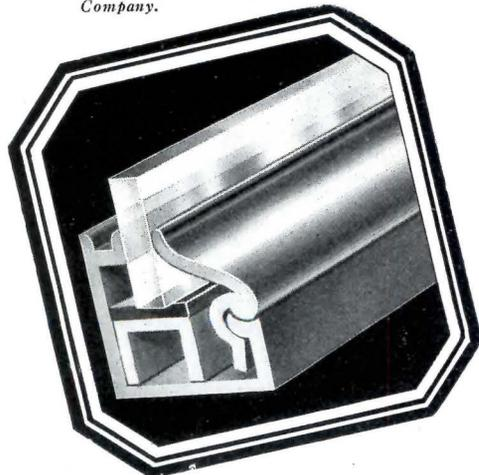
Showing the patented fulcrum principle used in all Davis sash and bars to assure safety to the plate. All glass is set from the outside without need for putty or plastic cement.
