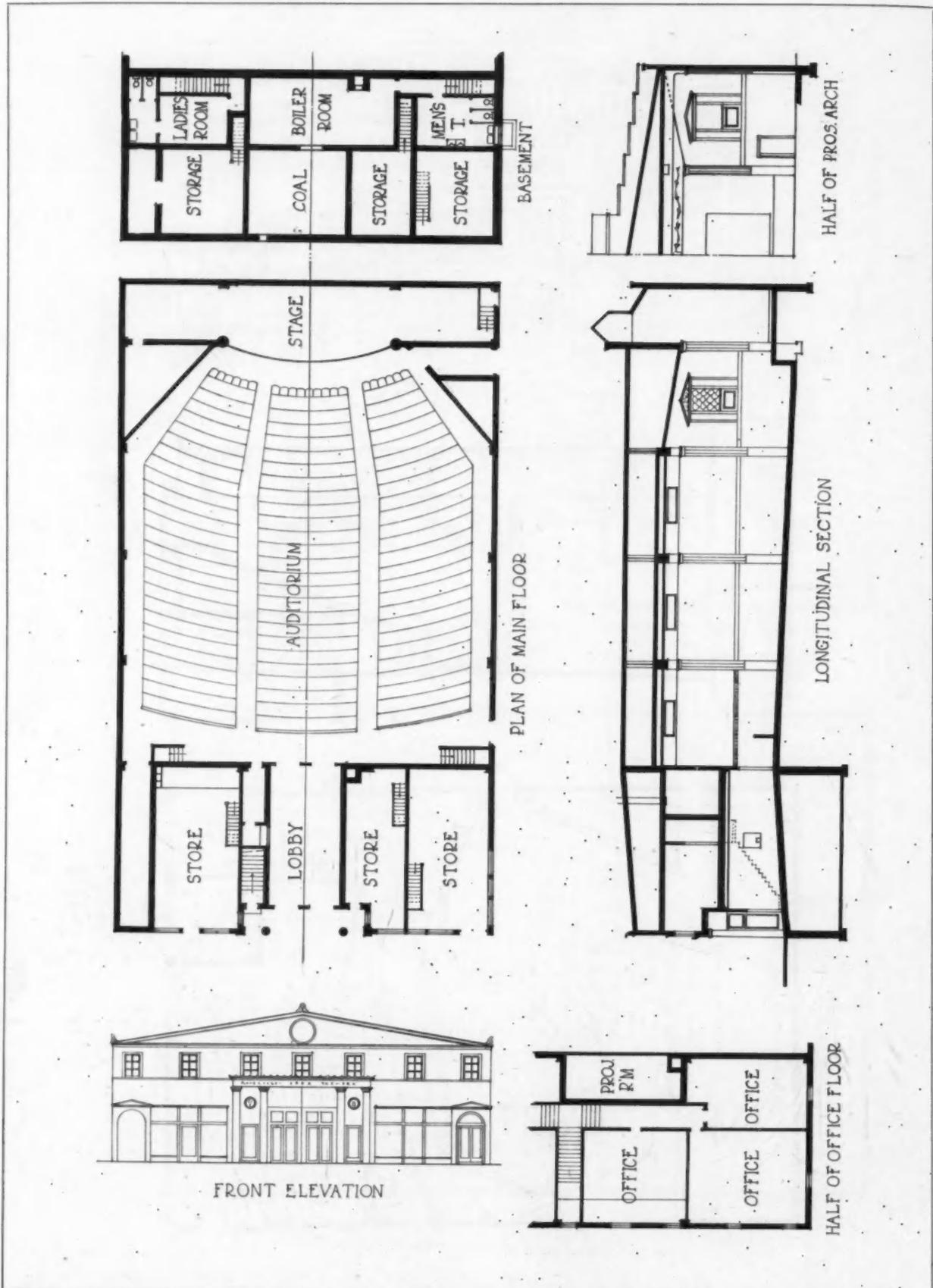
Elevation, Longitudinal Section, and Plans of the Basement, Main and Mezzanine Floors of a Motion Picture Theater for a Small Town
