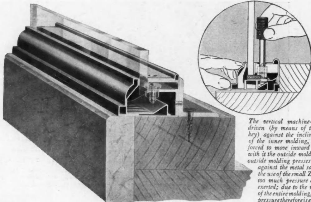
The vertical machine-screw is driven (by means of the Zouri key) against the inclined plane of the inner molding, which is forced to move inward bringing with it the outside molding. The outside molding presses the glass against the metal sash. With the use of the small Zouri key, too much pressure cannot be exerted; due to the movement of the entire molding, localized pressure therefore is eliminated.
