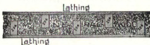
Section of Sound-Proof and Fire-Proof Partition
