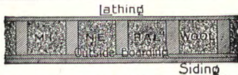
Section of Outside Wall of House, Showing Wool Between Studding
