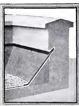
Metal Flashing Form with Flashing installed in concrete wall
