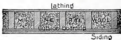
Section of Outside Wall of House, Showing Wood Between Studding
