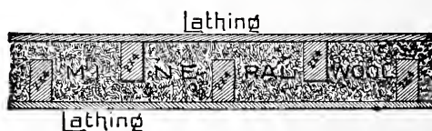
Section of Sound-Proof and Fire-Proof Partition
