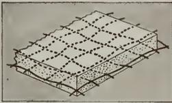
This is what usually happens to reinforcing mesh when a concrete mix having a low pourability is used.
