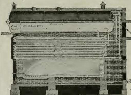
WITH many tubes in one header, the unequal expansion causes leaky joints. Rolling thins the tube ends and means new tubes. In the design of a header holding but two tube ends each tube can expand without strain on header or joints. This is another feature of the
