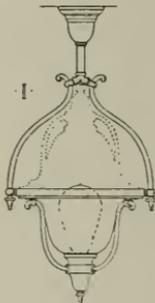
A fixture has been devised, the "Indirectirect,"\* to meet all these requirements and to admit of the utmost flexibility of treatment. The single unit type is of peculiarly interesting form (I) and is made in 100 watt, 150, 250, 400 and 500 watt sizes according to requirements. The multiple unit type (J) is not unlike the ordinary chandelier in form. Both
