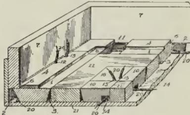
to facilitate the laying of electric wires. This strip is designated by the reference character 1, and has both its edges beveled or undercut, as shown in the illustration. A space is formed between one beveled edge and the wall for the reception of electric wires, 20, while the shape of the other edge, 3, permits the strip to be rotated about its lower outer edge in such a manner that it can be removed from its position, even though the edge of the base-board, 7, overlies it.
