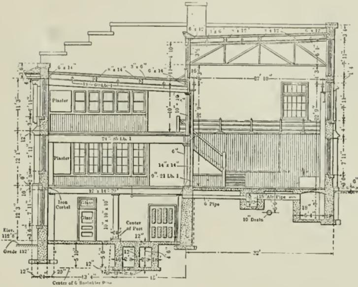
Fig. 4.—Cross-Section Through Machine Shop
