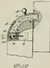
locking block (7) is urged by a spring (9) so as to hold the bolt (3) in the position shown in the illustration. The block (7) may be withdrawn by means of a key and the bolt (3) thus permitted to drop.
