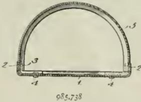
flanges (2) and an arch-shaped top (5). The edges of this top fit between the flanges (2) and L-shaped fastening members (3) bolted to the bottom plate.
