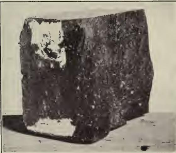
This Half Brick was subjected to over 150,000 pounds pressure, equal to 300,000 for the Whole Brick (15,000 per square inch); absorption test thirteen one-hundredth of one per cent. Test made by Engineering Department City of San Francisco.
