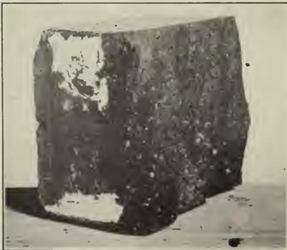
This Half Brick was subjected to over 150,000 pounds pressure, equal to 30,000 for the Whole Brick (15,000 per square inch) absorption test thirteen one hundredth of one per cent. Test made by Engineering Department City of San Francisco.
