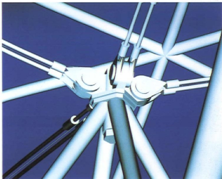
Computer generated perspective of one of the structural columns with details of the steel structural 'tree'
