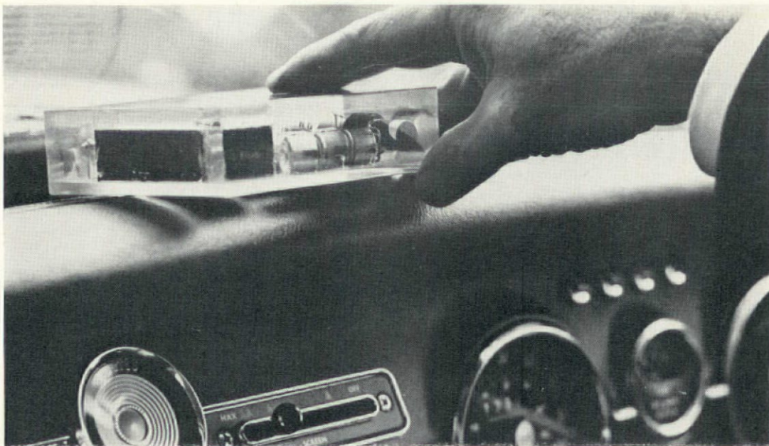
10, 11. Road pricing meters now under test at the Road Research Laboratory would require a motorist to 'pay as he drives'. The meter shown is actuated by passing over cables set at intervals in the road bed Photos: Topix
