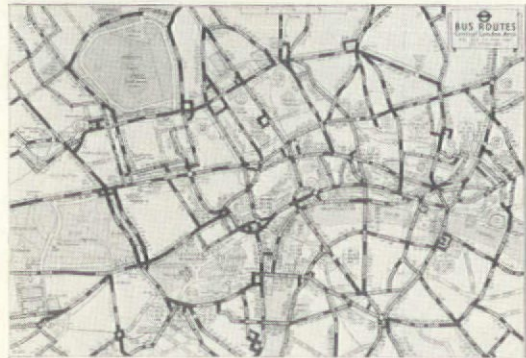
6. Bus map of central London, showing how a theoretically flexible system has, in fact, followed the main roads. Travel speeds at peak hours can be as low as 4 m.p.h., due to congestion
