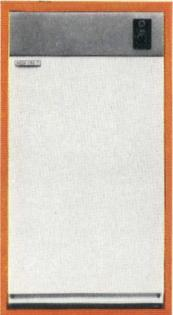
New departure in central heating: automatic and fully insulated 38,000 BTU/hr oil-fired kitchen boiler. Dimensions (36 in. high x 21 in. deep) and finish (stove enamelled steel sheet) match those of other kitchen units.
