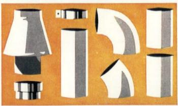
Modern Vitreous-Enamelling of steel components in H and V equipment, gives excellent resistance to corrosive fumes and products of combustion. Surfaces remain easily cleaned, hygienic, retain their good appearance. As the glass coating is fused onto the steel at 800°-900°C it also offers useful high-temperature resistance.
