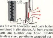
Gas fire with convector and back boiler combined in slim design. All front visible parts are number one finish EN-60 stainless steel, polythene wrapped during pressing. Aluminised steel is used for the heat exchanger.
