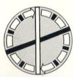
The unique, specially balanced pivot hinges of the Berkeley Double Glazed window permit it to traverse 180° and to be held securely at any angle within the arc. This affords maximum adjustability, provides any desired degree of ventilation and facilitates cleaning. Furthermore, the design of the hinge eliminates the possibility of wear impairing the functioning of the window.
