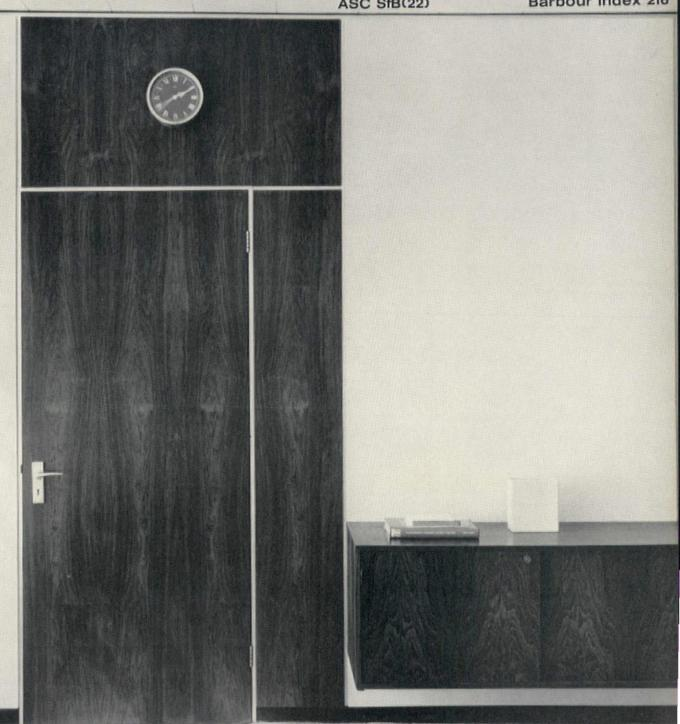
TENONFLEX executive partitioning creates a quality environment without the clumsiness of traditional building means. Panels veneered in matching timbers or wrapped in P.V.C. are secretly fixed to a polished aluminium frame—giving a recessed joint. Glass wool quilting ensures privacy and a sheet lead lining is available for accoustically critical areas.
