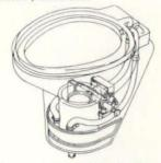
Left, the Tokaido train unit. The solids are broken down by an impeller and fed through a centrifuge from which the liquid is discharged outside the train Above and right, aircraft unit for DC 8, 707 and Caravelle. Push-button control for flushing spray, filters and pump. Solid particles are retained in the tank, liquid is mixed with disinfectants and recirculated
