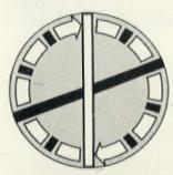
The unique, specially balanced pivot hinges of the Berkeley Double Glazed window permit it to traverse 180° and to be held securely at any angle within the arc. This affords maximum adjustability, provides any desired degree of ventilation and facilitates cleaning. Furthermore, the design of the hinge eliminates the possibility of wear impairing the functioning of the window.
