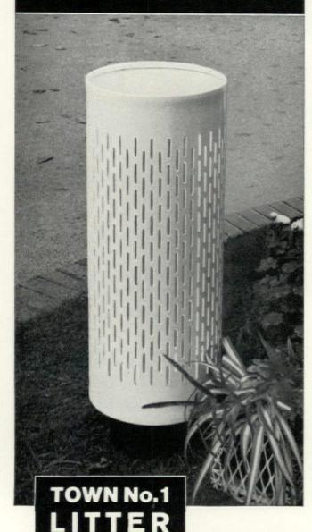
Winner of a Design Centre Award, this bin is ideal for public squares and shopping areas. Perforated steel body with dished bottom for added strength. Easily removed from base for emptying, simple locking device prevents unauthorised removal. Standard finish: body covered white polythene plastic, base galvanized and stove enamelled black. Size 2' 6" high x 101 dia.
