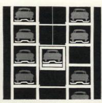
Vertical 'Keypark' Fully automatic' steel-pallet/high-speed lift system meets high-density parking needs. Rust-proofed, pre-fabricated steel frame structure employs standard modular units. This system's ability to increase the car parking capacity of a small site, measuring only 24 ft x 22 ft, by up to 1,000 per cent, makes 'Keypark' especially practical where land values are high. Can also be installed integrally within buildings.
