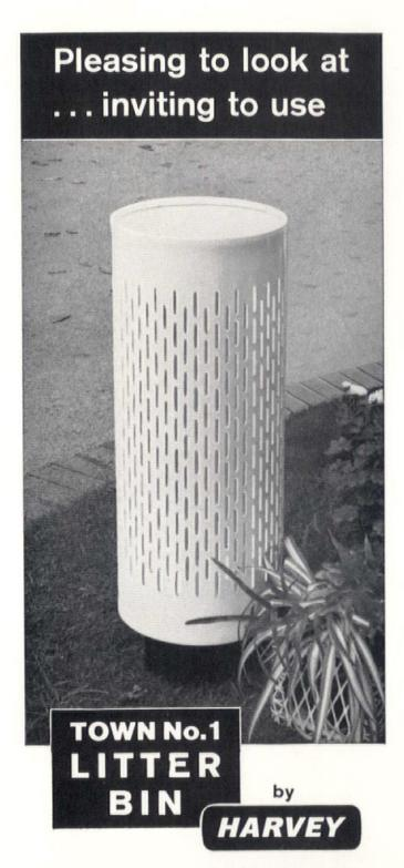
Winner of a Design Centre Award, this bin is ideal for public squares and shopping areas. Perforated steel body with dished bottom for added strength. Easily removed from base for emptying, simple locking device prevents unauthorised removal. Standard finish: body covered white polythene plastic, base galvanized and stove enamelled black. Size 2' 6" high x 101 dia.
