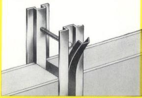
Detail showing construction of partition using aluminium sections and hardboard-faced Stramit-core panels. Note plastic-insert which conceals bolt-heads.
