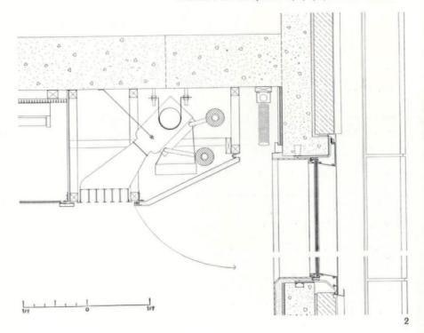
1. A perimeter air-conditioning ring which houses standard 'Velovent' units inside white pressed metal casings (outside this there are electrically-operated venetian blinds on S.E. and S.W. faces).
