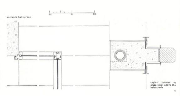
aluminium is fixed by galvanized steel brackets bolted to the reinforced concrete and there are cast aluminium junction pieces between units,
