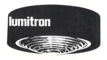
Universal drums and recessed units with interchangeable louvres, lenses and opal glass diffusers. The drums are available as ceiling or pendant fittings with matching wall brackets in 3 sizes and the recessed units in 2 sizes — all taking 100-200 watt lamps. Constructed in aluminium and permanently finished in anodised silver, gold, copper or stove enamelled colours.
