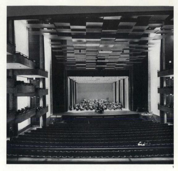
View of auditorium showing part of the pit raised to stage level; also the suspended ceiling which acts as acoustic reflector
