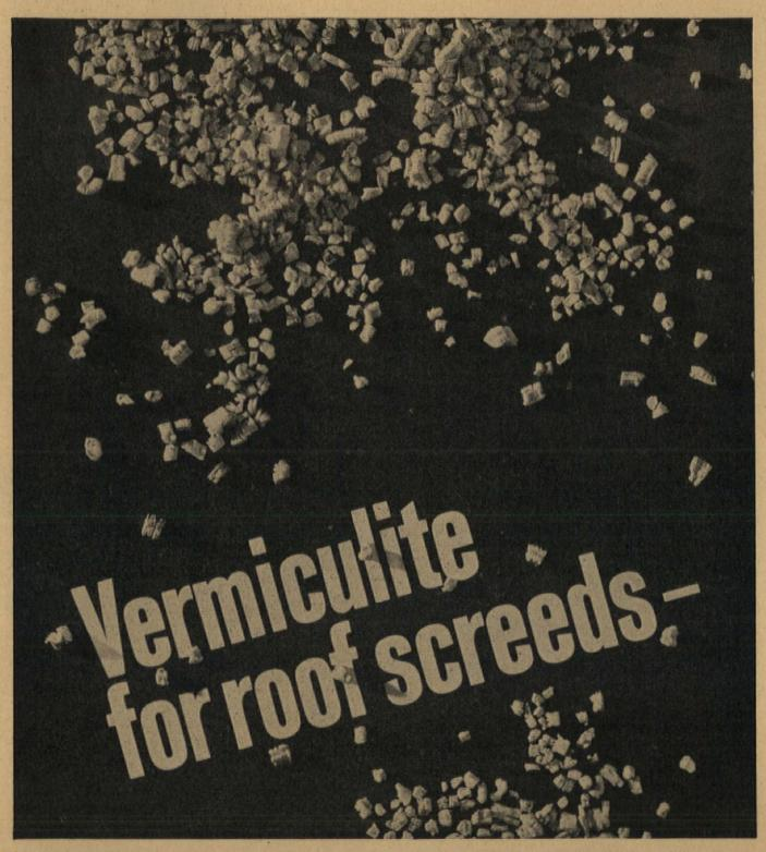
\* Density 22-26 lb/cu. ft. with 'k' value 0.63-0.75 B.Th.U. \* Highest resistance to fire \* Permanent, jointless, non-warping base for all finishing materials \* Stable aggregate \* No special equipment needed for mixing or laying \* Very easy to lay, even on steepest slopes.
