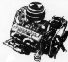
**Efficient High Torque 283 V8**—made to order for runs that call for the extra punch of V8 power. Advanced short-stroke design knows how to nurse extra power and miles out of every drop of gas. 160 hp and 270 ft.-lbs. of torque get big loads moving quickly and efficiently. Top durability features include chrome-plated piston rings, Moraine 100 bearings and hydraulic valve lifters.
