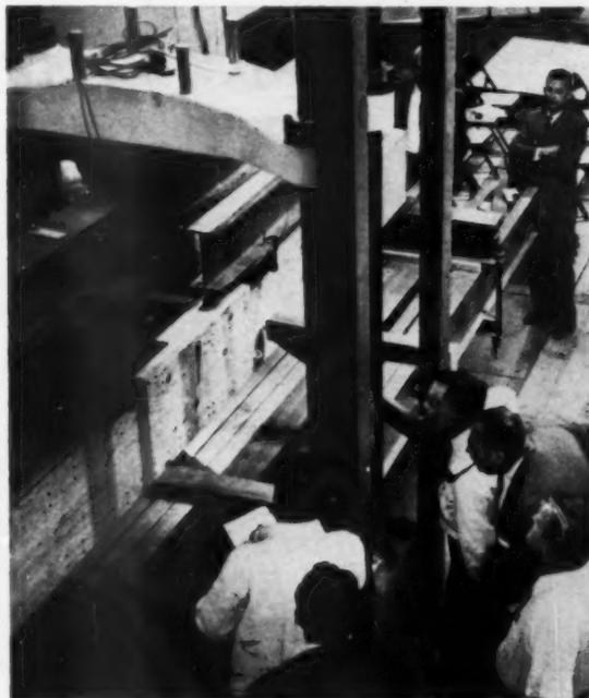
**DFPA ENGINEERS** and NAHB technical committee watch a test of nailed-only header. It took  $2\frac{1}{2}$  times design load.
