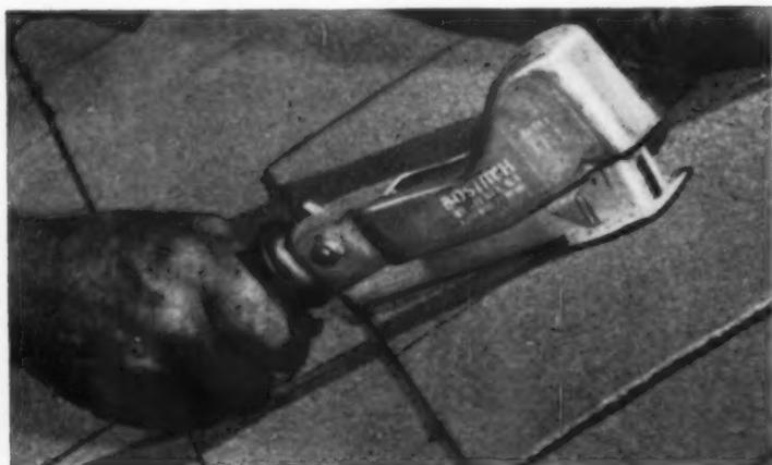
Why? Because applying asphalt shingles with the Bostitch H4 Stapling Hammer is as much as four times faster than with hammer and nails, giving you time to do more jobs.
