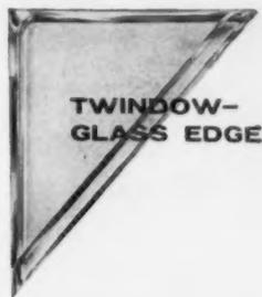
**TWINDOW—GLASS EDGE.** This type is just the thing for modern window-wall construction. Having exceptional insulating properties, it is constructed of two panes of  $\frac{1}{8}$ " PENNVERNON®—the quality window glass—with a  $\frac{1}{16}$ " air space between. TWINDOW glass edge units are available in popular sizes for a variety of window styles.
