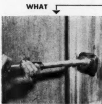
**APPLICATIONS UNLIMITED** . . . Powder-actuated "Drive-It" nails almost anything onto concrete or steel.
