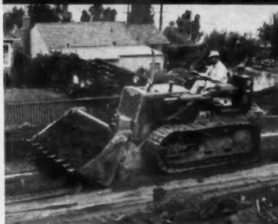
As "carry-type scraper" this TD-9 4-In-1 gives inch-close lot-grading accuracy, spreads with precision. Close-coupled, this unit delivers its big capacity where "long hitched" outfits can't profitably maneuver. "The 4-In-1 gets me jobs an ordinary loader can't begin to do," states Owner Harold Swanson, Richmond, Calif. "My competitors are buying 4-In-1's to equal what I can do!"
