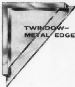
**TWINDOW—METAL EDGE.** This type is ideal for large windows and where maximum insulation is needed. It's made up of two panes of  $\frac{1}{8}$ " clear-vision Plate Glass, with a  $\frac{1}{2}$ " sealed air space between. Its stainless steel frame, a TWINDOW feature, eliminates bare edges . . . makes handling safe, quick and easy.
