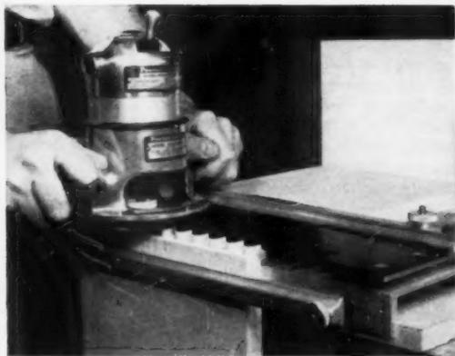
A real selling extra for home builders—dovetailed drawer joints. Quickly and accurately cut with Porter-Cable Router and precision Dovetail Templet.
