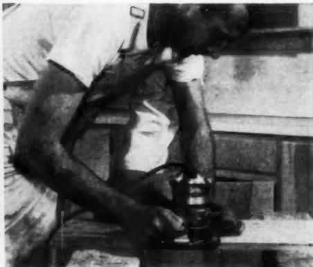
With over 150 available bits and cutters, tremendous variety of edge mouldings are possible. Corner round and standard  $\frac{3}{8}$ " rabbet cuts for cabinet doors are each made in one pass with Router.
