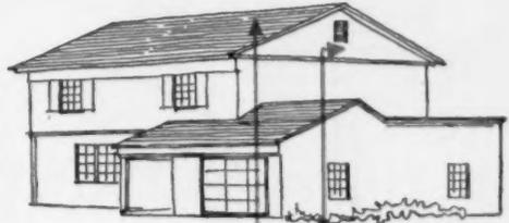
"Replacing the hip roof with a gabled roof, and using horizontal siding on all sides, would make the house seem larger. And the gables would permit installation of ventilating louvers at each end."
