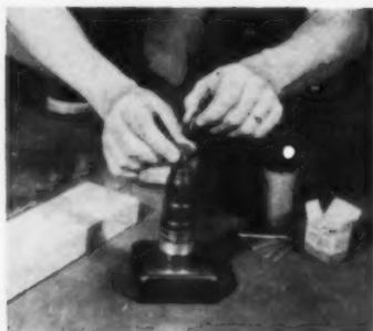
2. NAIL is dropped into barrel, then power load is inserted into tool.
