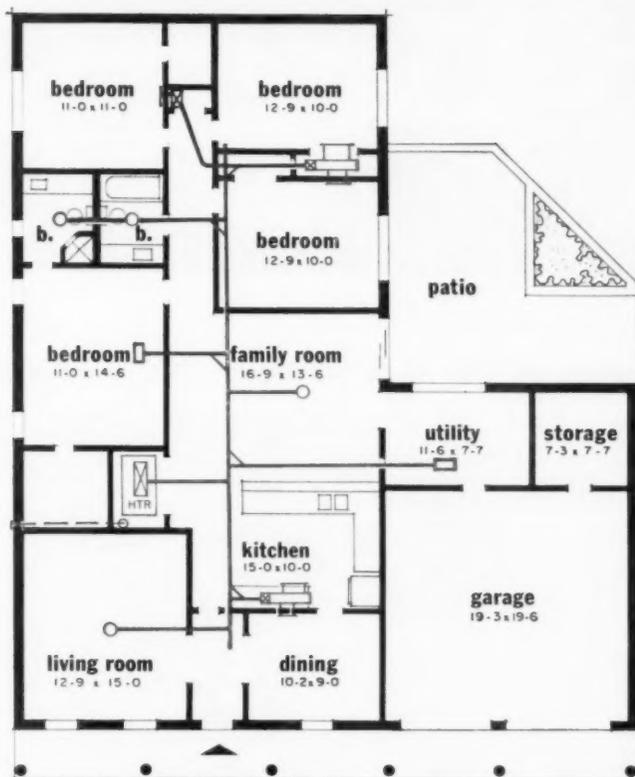
**DUCTWORK LAYOUT** was also engineered for Dobbins by United Gas Corp. To hold costs down and make the equipment as efficient as possible, the main equipment is placed at a mid-way point in the house. Evaporator cooler was stationed in the yard.
