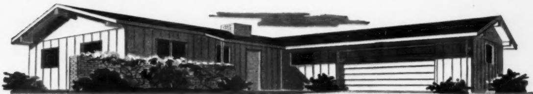
**BOARD AND BATTEN** styling with tough, abrasion-resistant Duraply's CreZon overlay to help prevent moisture penetration, control checking and swelling, and eliminate paint peeling. Duraply needs no sanding, and just two coats of a quality exterior paint last for a minimum of five years before repainting is needed.
