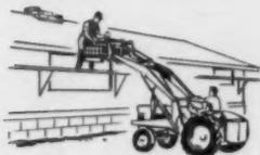
① **PALLET FORK** handles brick, block, lumber, roofing, large materials.
