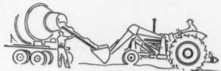
**YOU CAN CARRY** concrete in the loader bucket and dump it into places that the ready-mix concrete truck can't reach. This is much faster and cheaper than hand-trucking the material in wheelbarrows.
