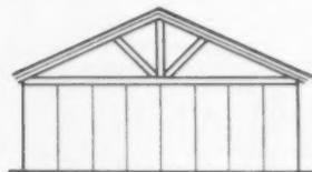
Beamed-ceiling construction (slope 2" in 12")
