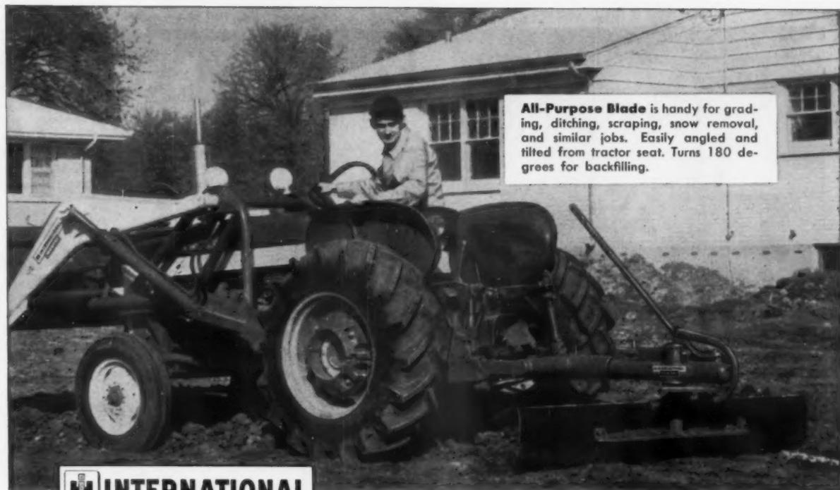
**All-Purpose Blade** is handy for grading, ditching, scraping, snow removal, and similar jobs. Easily angled and tilted from tractor seat. Turns 180 degrees for backfilling.
