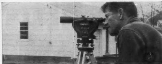
**MASTER BUILDER CONVERTIBLE TRANSIT-LEVEL.** Big instrument performance at a moderate price. Fast, accurate laying out of horizontal and vertical angles, leveling, plumbing, with horizontal circle and vertical arc and verniers. Rugged instrument yoke frame. 22-power internal focusing telescope; coated optics; 3-ft. short focus. Model 320 with stiff-leg tripod and field case \$229.50
