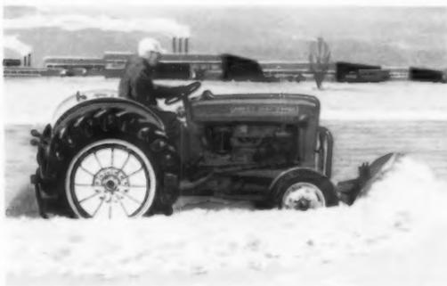
**SNOW REMOVAL**—With Select-O-Speed you have easy shifting to powerful low gears for big drifts, and to higher, fuel-saving gears when the going is easy. Extra safety is at your finger tips, too, with Select-O-Speed brake assist for stopping on ice.
