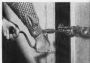
Bit guide remains in same position for drill edge hole and guiding bit in making perfectly aligned hole. Kit has hand or power bits.
