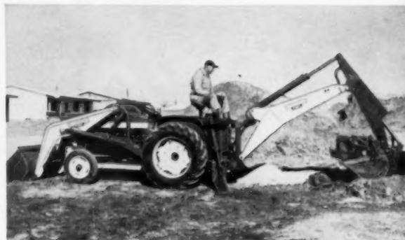
**Three 6-cylinder power ratings, 61 to 90 gross engine hp—** all available with gasoline, Diesel or LP Gas engines. Above, the 61 hp International 460 Utility with International Wagner backhoe and loader.
