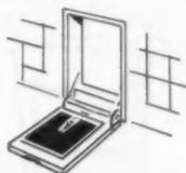
**BUILT-IN SCALES:** Fits into bathroom wall recess. Housing for unit is roughly 14" x 23", with outside dimensions, 16" x 25". Lowers to floor on spring.
