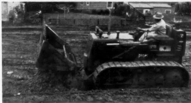
He can grade with accuracy using 4-in-1 "carry-type scraper" action to let the dirt boil in. With this same action he can strip sod; skim-off layers of materials. And he can regulate clam lip opening to spread materials precisely!
