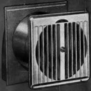
Gives automatic through-the-wall ventilation. Powerful pressure blades exhaust odors and vapors outward and downward. Weather tight damper opens and closes automatically. Model 888A (illustrated) has remote switch - Model 889A is chain operated.
