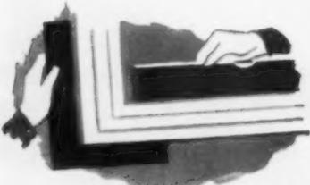
Check window opening to make sure it is square, level and has sufficient clearance.
