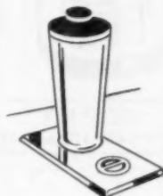
**FOOD CENTERS:** Installs so that power unit is below surface of counter. Connects to 115-volt AC outlet. Generally has six speeds. Is sold with or without its attachments, which include a mixer, blender, fruit juicer, knife sharpener, and meat grinder.
