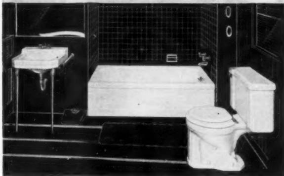
**Catalina Economy Bathroom**, designed and built for The Mighty Middle. Gerber packaged bathroom No. 3. Ledge-type lavatory, No. 310, 19" x 17", has concealed front overflow and centerset faucet, No. 141. Closet is close-coupled, washdown type, 12" rough-in, No. 900. Porcelain enameled steel recessed tub, No. 006, with connected waste and overflow, No. 189GB, and over-the-rim tub filler No. E480.
