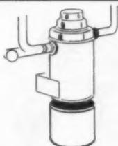
**BUILT-IN VACUUM SYSTEM:** Canister and power units are generally installed in basement, garage, closet or utility room. Ducts run under floors, between studs. Three to five outlets are sufficient for the average home. Units vary from 2/3 HP to 1 1/2 HP. Operates on 115 Volt, 60 Cycle current.
