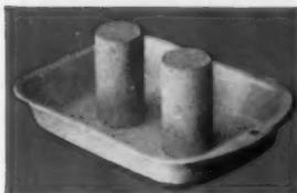
To compare the durability of Brixment with that of ordinary cement-and-lime mortar, make a cylinder of each, let both cure for a month, then freeze and thaw them 40 or 50 times with a little water in the pan.
