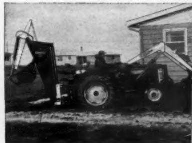
**35 hp International 330.** New and real rugged! Has the built-in 'beef' to handle 1,000 pounds with front-end loader; step up yardage with choice of heavy-duty backhoes that maintain grades, digging 10 or 12-ft ditches.
