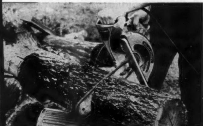
**THE CIRCULAR HAND SAW**, pictured here with a chain saw attachment, is placed at the top of the list when it comes to time-saver tools. The bayonet saw, sabre saw and chain saw also rated high on builder's lists. Above, a Black & Decker model (No. F57, p. 124).
