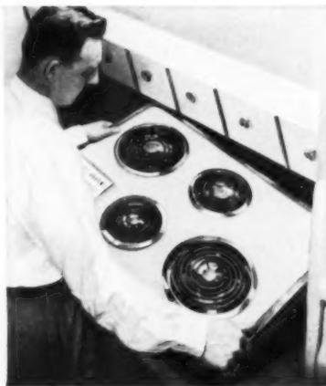
One-piece drop-in cooktop has built-in pushbutton controls . . . is easy to install. Drops into 29 13/16" x 20 7/16" opening . . . fits flush into countertop with accompanying sink-rim flange trim.
