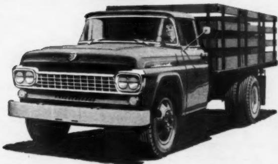
**FORD MEDIUM DUTY TRUCKS** (F-600 shown) available with 9- or 12-ft. stake bodies, offer wide choice of modern Short Stroke power, V-8 or Six. 1½- or 2-ton models with GVW's from 15,000 to 19,500 pounds. Fully automatic Transmatic transmission available.
