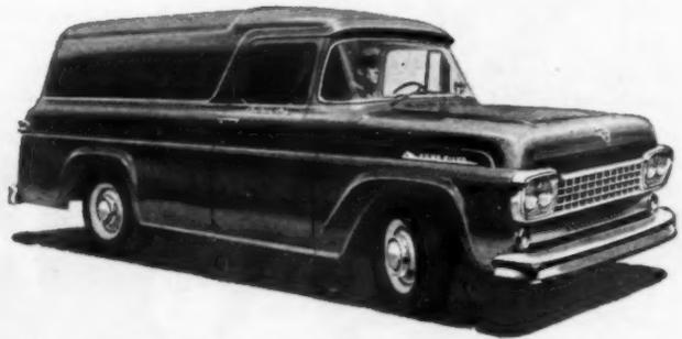
**FORD F-100 CUSTOM PANEL** features roomy, all-steel, fully lined body. A big 158 cubic feet of loadspace and wide rear door opening easily accommodates bulky articles. Its 110-inch wheelbase makes it highly maneuverable in traffic.
